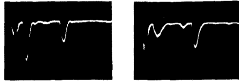
A. GROUNDWAVE, E LAYER (320 \mu s) AND F LAYER (900 \mu s) PULSES. B. GROUNDWAVE, ONE HOP E LAYER (350 \mu s), TWO HOP E LAYER (700 \mu s) AND F LAYER (900 \mu s) PULSES
