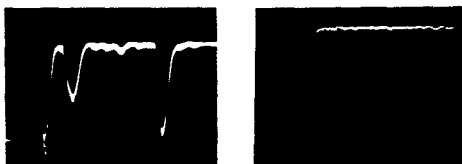
A. GROUNDWAVE, E LAYER (360 \mu s) TWO HOP E LAYER (700 \mu s) AND F LAYER (1100 \mu s) PULSES. OCT. 28, 1958 B. GROUNDWAVE PULSE ONLY NOV. 5, 1958
