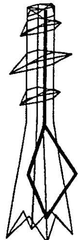
Figure 3 Double-Elbow Stub on one tower leg
