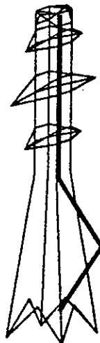
Figure 2 Elbow Stub on one tower leg
