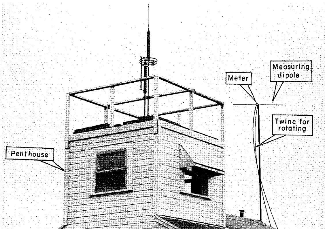
Fig.7.— Transmitting antenna showing receiving dipole used to measure the relative field intensity and polarization in the horizontal plane.
