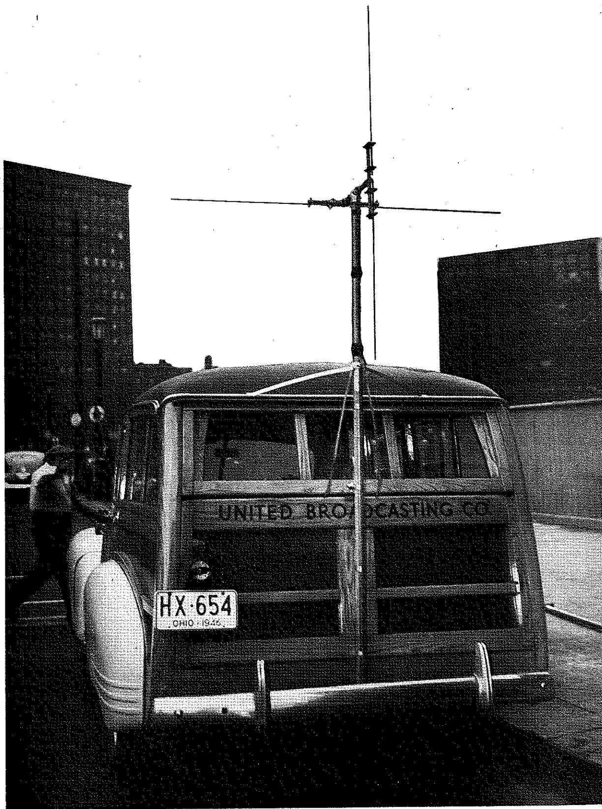
Fig. 18.—Antennas for simultaneous reception of vertically and horizontally polarized waves.
