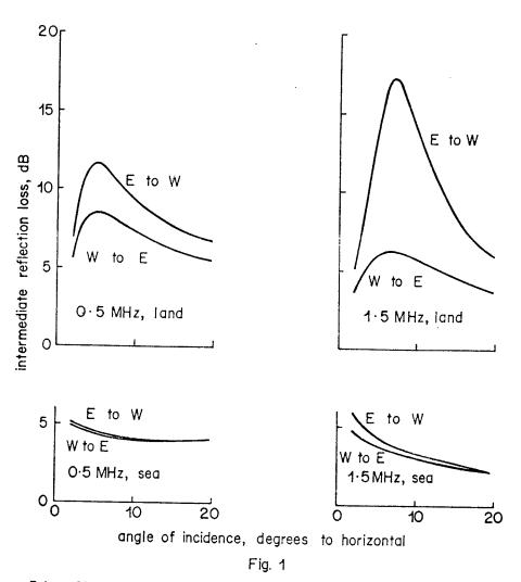
Intermediate reflection loss on east-west paths at 65° dip latitude
