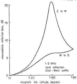
Fig.2 Variation of intermediate reflection loss with magnetic-dip latitude
