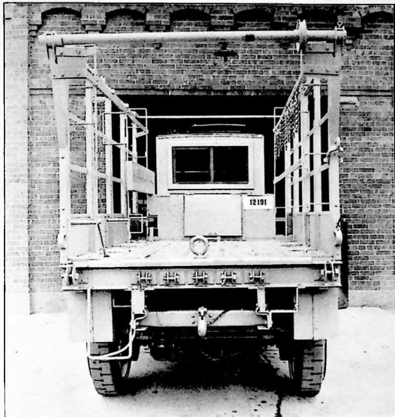
Rear view of the 2½-ton Model 51 White truck and "C" type body
