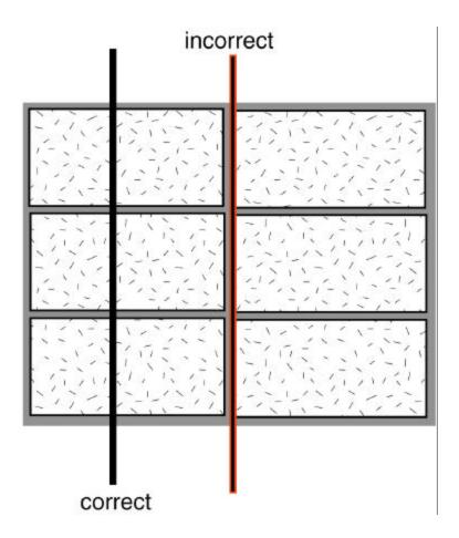
When installing in a drop ceiling also note that there may be other substantial metal items in the area. This may include HVAC ducts, water pipes and metal conduits. It is important to avoid placing these items between the users and the radiating cable as they may cause attenuation. Do not attach the cable directly to these items, and attempt to make any crossings of these items in a perpendicular manner.
