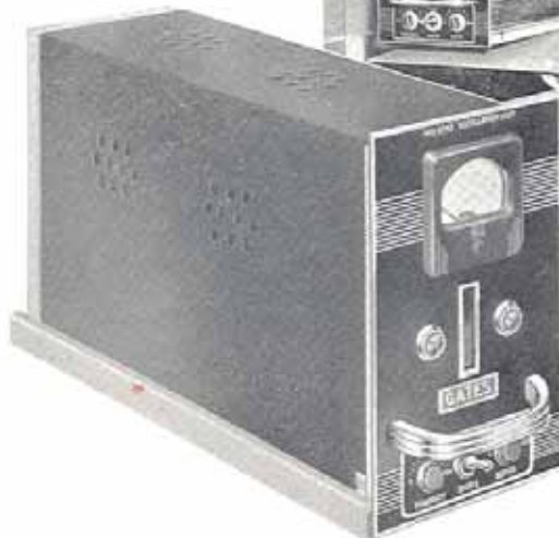
At the left is shown one of the frequency control units removed from the transmitter. Each one contains a complete oscillator and first buffer with crystal and oven. The thermometer on the crystal oven can be viewed thru the vertical slot on the front. Tuning controls and switch for changing the meter from the plate circuit of the oscillator to that of the buffer are located at the bottom of the panel.
