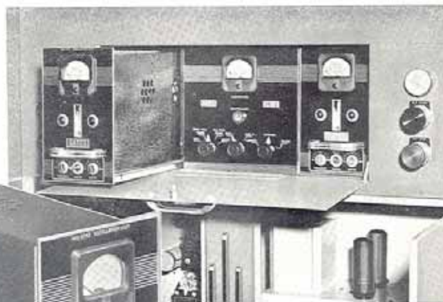
Above is the "Customaire" showing front doors open and wide accessibility to tubes and relays. At the right is a close-up of the frequency control unit section. On the center panel are the tuning controls for the entire transmitter.
