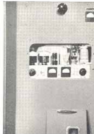
Oscillator and first intermediate amplifier with front slip-on cover removed. Entire unit can be removed in 8 seconds for servicing.
