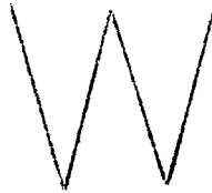
Fig. 9, Typical Waveform, Output V104 (first section)
