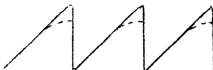
Fig. 7, Typical Waveform, Output V103 (V104 removed).
