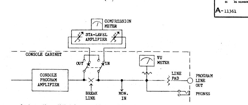
Almost any console is easily modified for use with Gates' STA-LEVEL Amplifier as shown above. Simply remove the output from the console program amplifier, as shown by the break, and connect to the input terminals of the STA-LEVEL Amplifier. Connect the output of the STA-LEVEL Amplifier to the output circuit of the console. The use of a console utility switch, or an external switch, will allow the STA-LEVEL Amplifier to be switched in or out of the circuit as desired.
