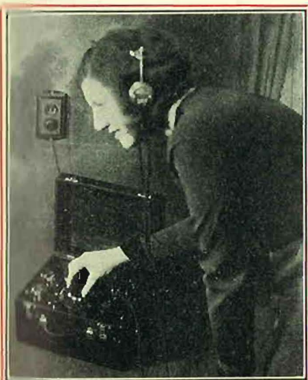
The individual receiver with two tubes, fully a-c. operated, provided with headphones.
