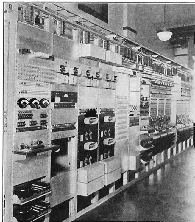
Fig. 8. Equipment for one terminal of 24-channel system.
