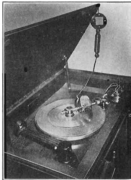
Accessory type of home recording equipment, using mechanical feed for tracking stylus.
