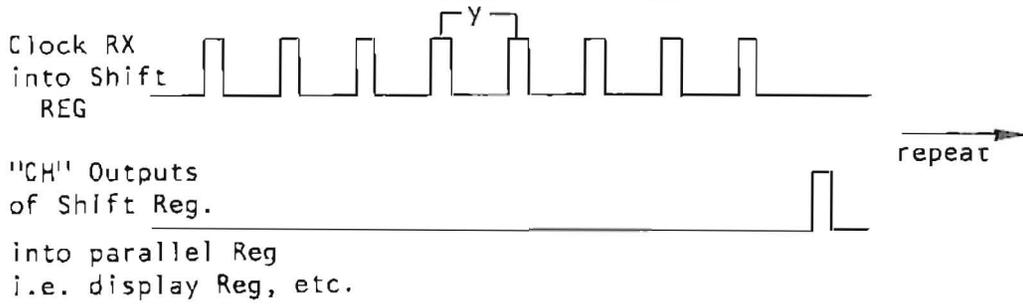
NOTE: There are eight y times during a complete XMIT or REC Cycle. During each y time the UART is sending or Receiving serial data as follows:
