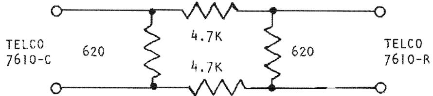
For microwave Uplink (STL) operation and FM Radio Downlink (SCA) operation:
