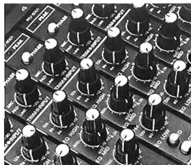
3-band variable frequency equalizer
