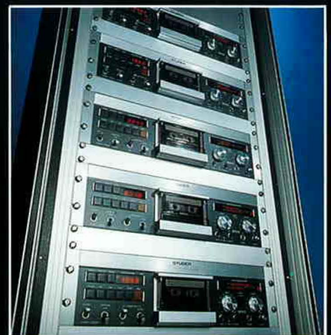
STUDER A710 recorders are prepared for 19" rack installation
