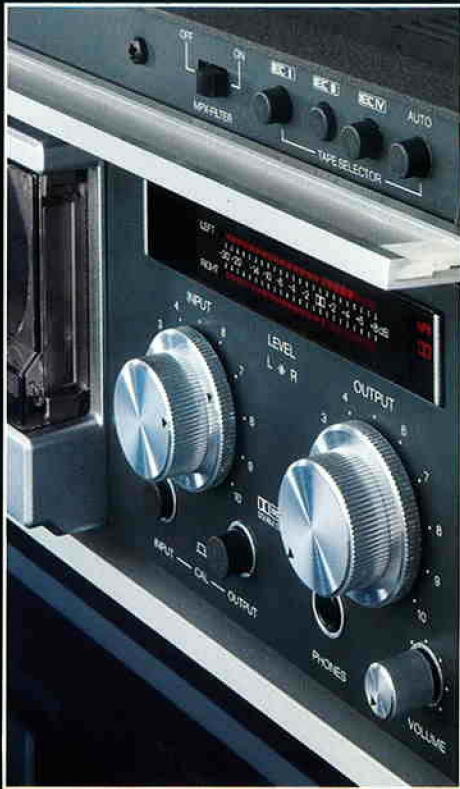
Closely grouped audio controls: tape bias selection according to IEC standards, potentiometers and push buttons for input and output level as well as headphones level.
