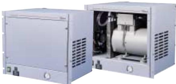
The **MT-600** series automatic membrane dehydrators are designed to provide the same features and benefits to large microwave and broadcast applications as the smaller MT300. They are equipped with the unique Andrew uni-mount system allowing for rack, wall or free-standing mounting without additional parts and are designed to supply dry air at a dewpoint of -45°C (-50°F), or better, under the ambient conditions of 95% RH at 49°C (120°F).
