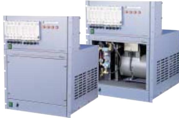
The **XT-1700 series** automatic membrane dehydrators are the largest rack-mountable units offered by Andrew. They are equipped with the unique Andrew uni-mount system allowing for rack, or free-standing mounting without additional parts. They are designed to supply dry air at a dewpoint better than -45°C (-50°F) under the ambient conditions of 95% RH at 49°C (120°F).
