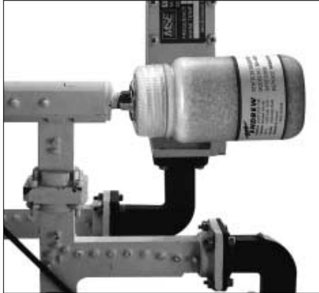
Static Desiccator SD-002A attached to 2 Port Combiner of 4.5 m ESA.
