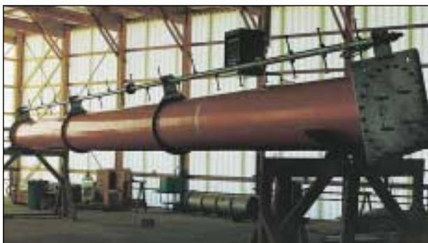
GUIDELINER antenna for WTIU channel 30 undergoing inspection.
