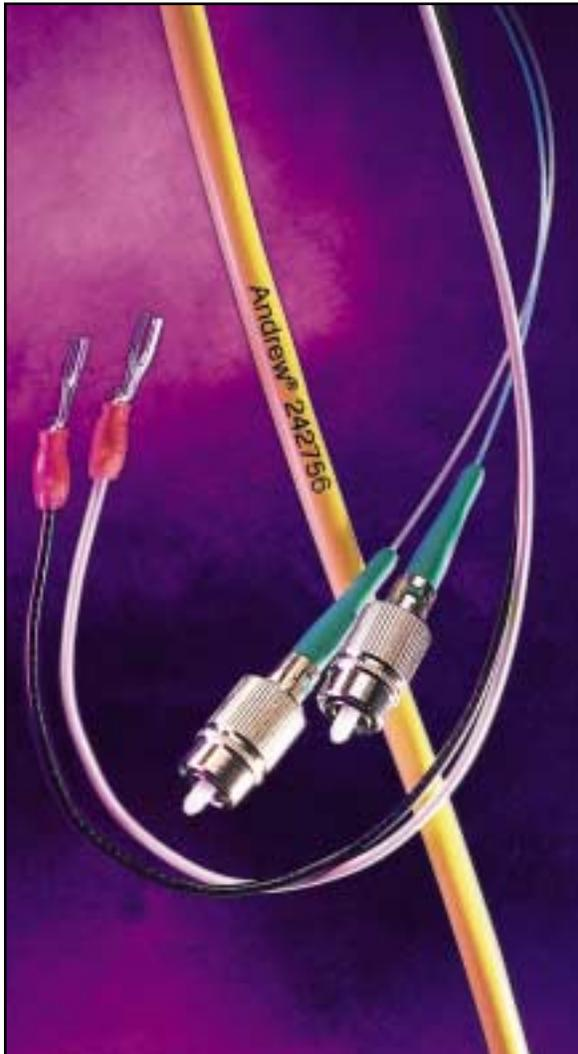
Andrew indoor composite cables combine two Andrew Microcable™ elements with two insulated copper conductors to provide electrical current and fiber optic capability in one cable. This plenum rated cable is ideally suited to indoor antenna remoting for cellular and PCS systems and for communication and sensor systems in industrial environments.
