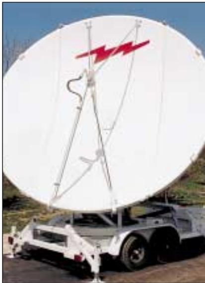
4.5-Meter Transportable Antenna
