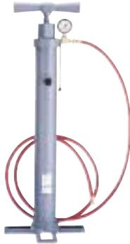
**Hand pumps** are lightweight portable air drying systems capable of pressurizing up to 30 lb/in<sup>2</sup> (210 kPa). Removal of moisture is accomplished by passing ambient air through a cylinder of color indicating silica gel desiccant. The pump contains a sight glass to view the moisture condition of the desiccant. When the dark blue color changes to amber, it is time to replace or regenerate the desiccant. Do not use the pump after the desiccant turns amber.
