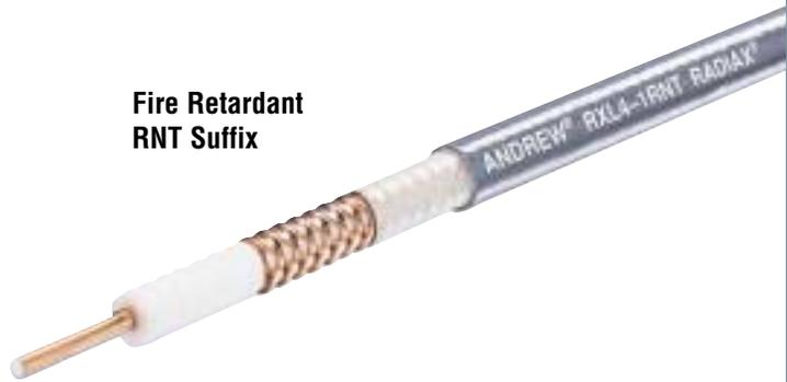
**Barrier Tape.** RNT suffix cables include a double mica barrier tape under the jacketing. This gives additional protection over the RNT1 suffix type cables. The tape is an inert material that does not burn or melt. In the event of a fire, the tape prevents molten dielectric material from flowing out of the slots and igniting.
