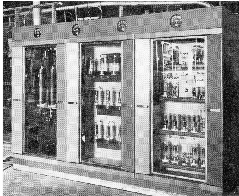
Figure 2—Three unit assembly associated with each 500 KW transmitter; (left) 15 KV rectifier tube assembly, (center) 3 bias rectifiers, (right) audio and RF driver.
