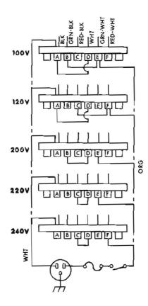
Fig. 3.7 Modifying AC Mains Voltage
