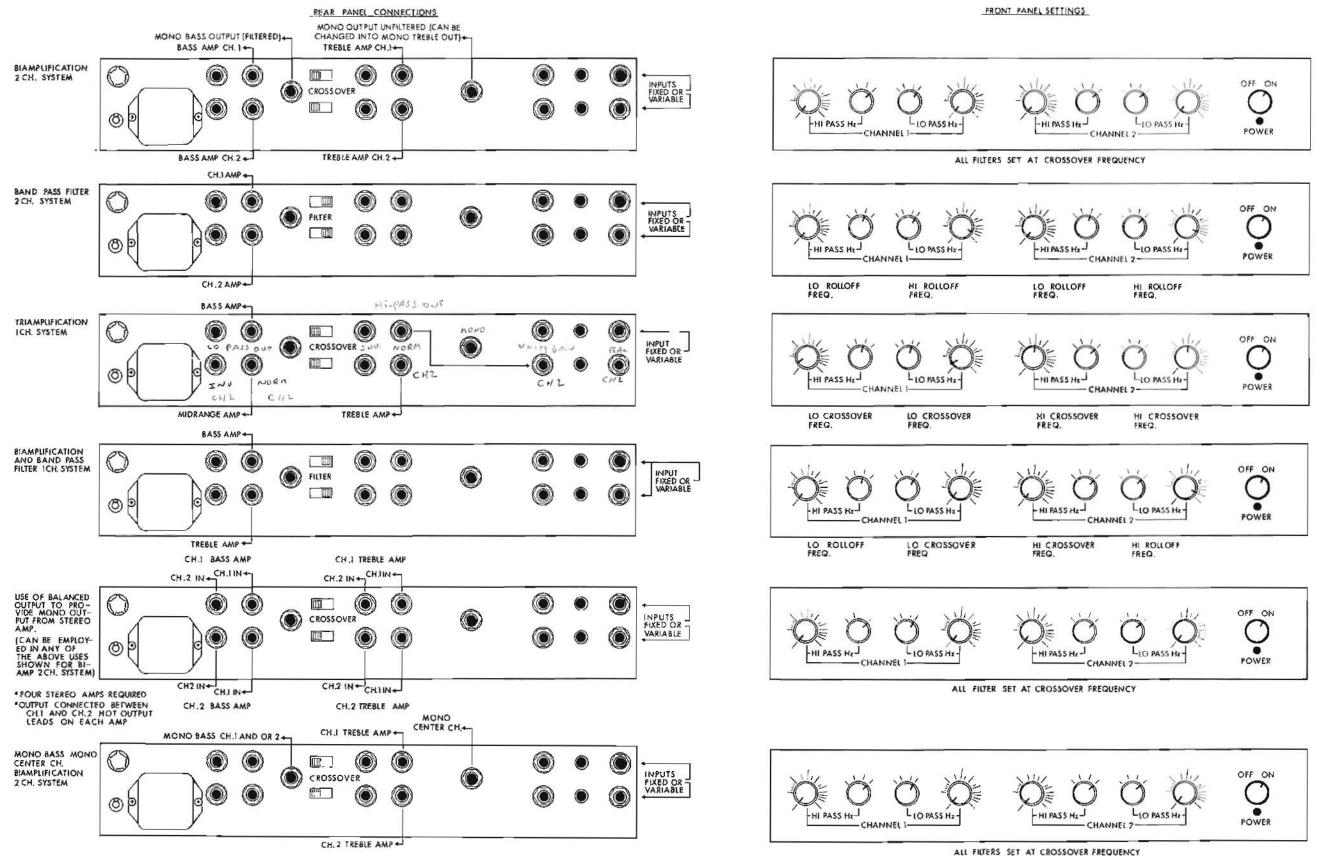
Fig. 3.2 Typical System Configuration and Cables
