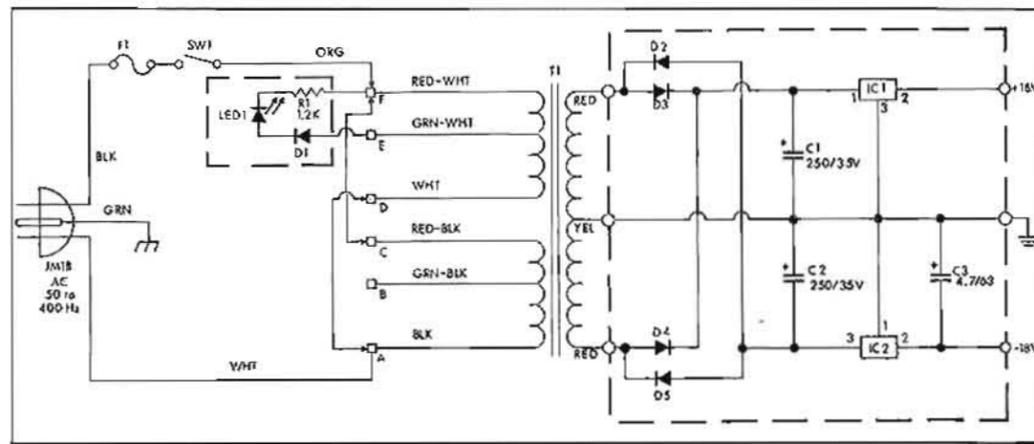
POWER SUPPLY SHOWN WIRED FOR 120 VAC. FOR OPERATION AT ANOTHER LINE VOLTAGE, FOLLOW CONVERSION CHART BELOW. SELECT THE CORRECT VOLTAGE: CAREFULLY IDENTIFY ALL WIRES BEFORE PROCEEDING. THE SIX TRANSFORMER PRIMARY WIRES ARE SOLDERED TO AN ADJACENT TERMINAL STRIP, (A, B, C, D, E, and F). ONLY FOUR WIRES ARE USED IN ANY CONFIGURATION.
