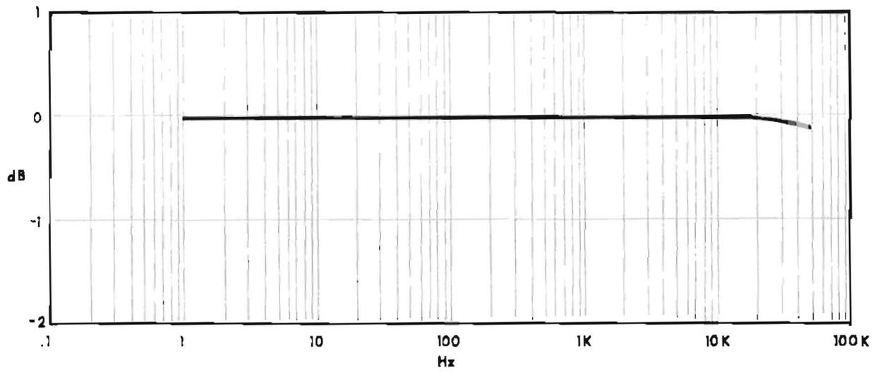
*Fig. 2.1 Typical Frequency Response:
