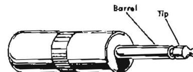
Fig. 3.4 Phone Plug,  $\frac{1}{4}$ ", 2 Conductor
