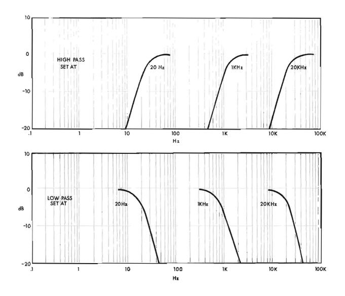
Fig. 2.4 Typical Filter Curves
