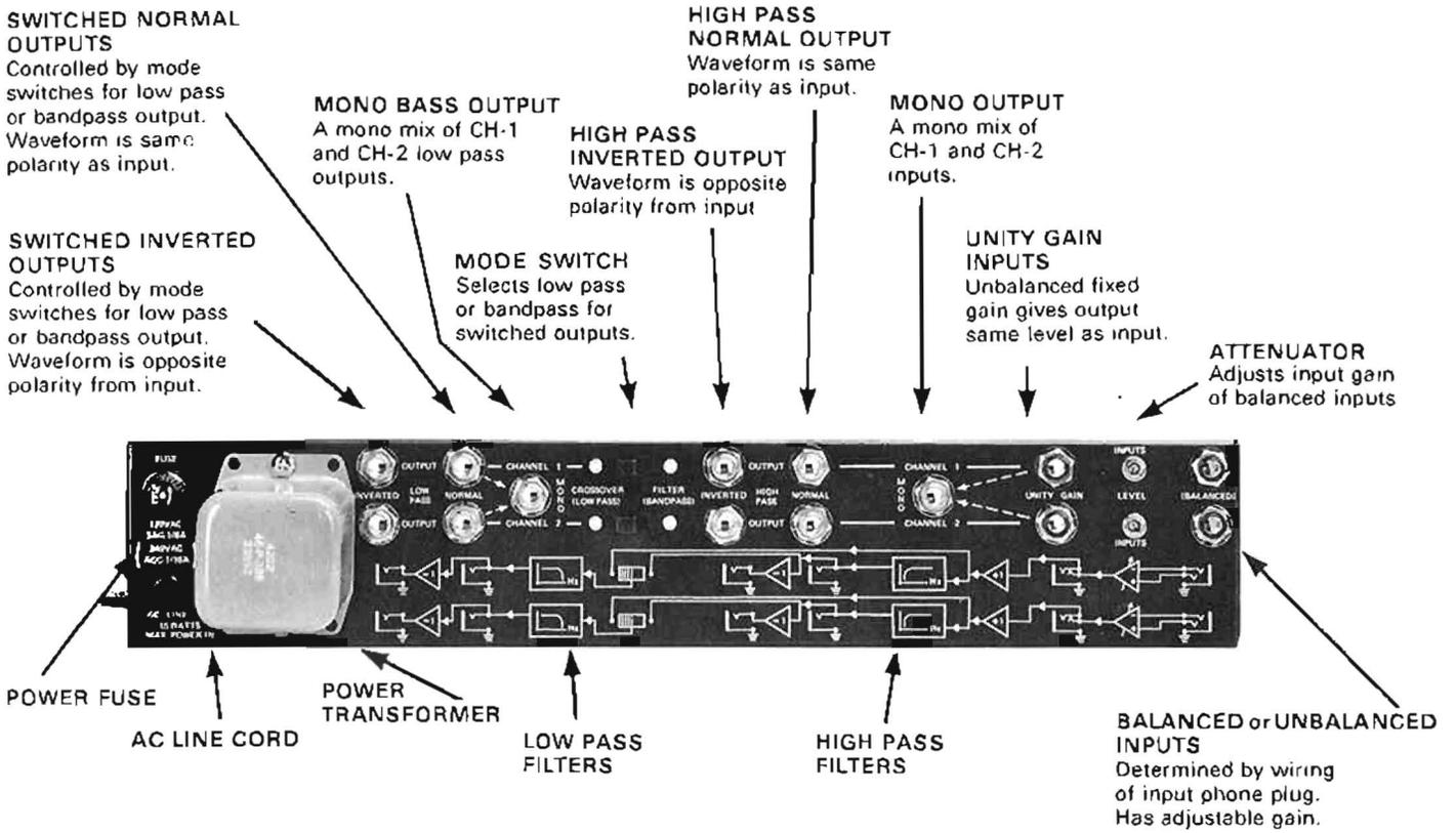
*Fig. 3.6 Rear Panel Controls and Connectors*
