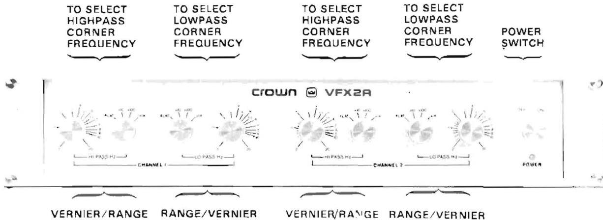
*Fig. 3.5 Front Panel Controls*
