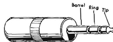
Fig. 3.3 Phone Plug,  $\frac{1}{4}$ ", 3 Conductor
