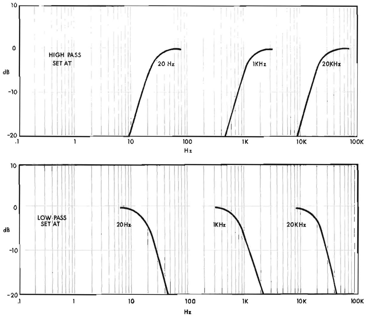
Fig. 2.4 Typical Filter Curves
