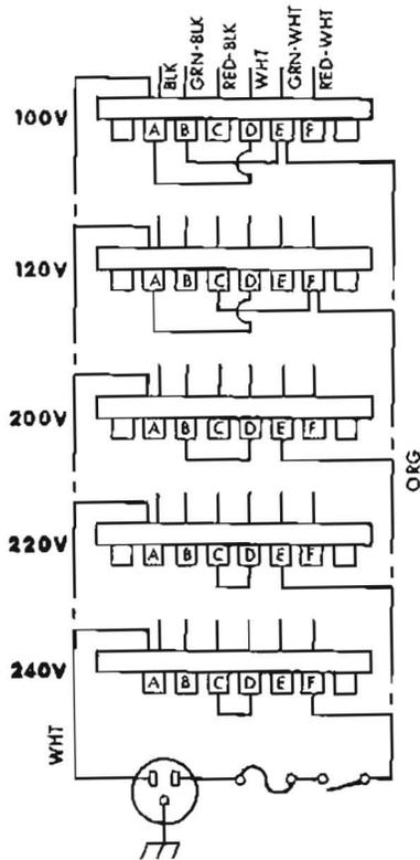
*Fig. 3.7 Modifying AC Mains Voltage*
