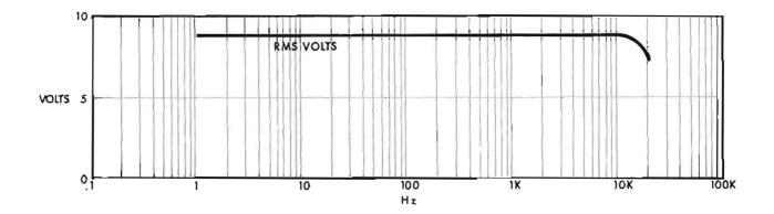
Fig. 2.5 Typical Maximum Output: IHF Load
