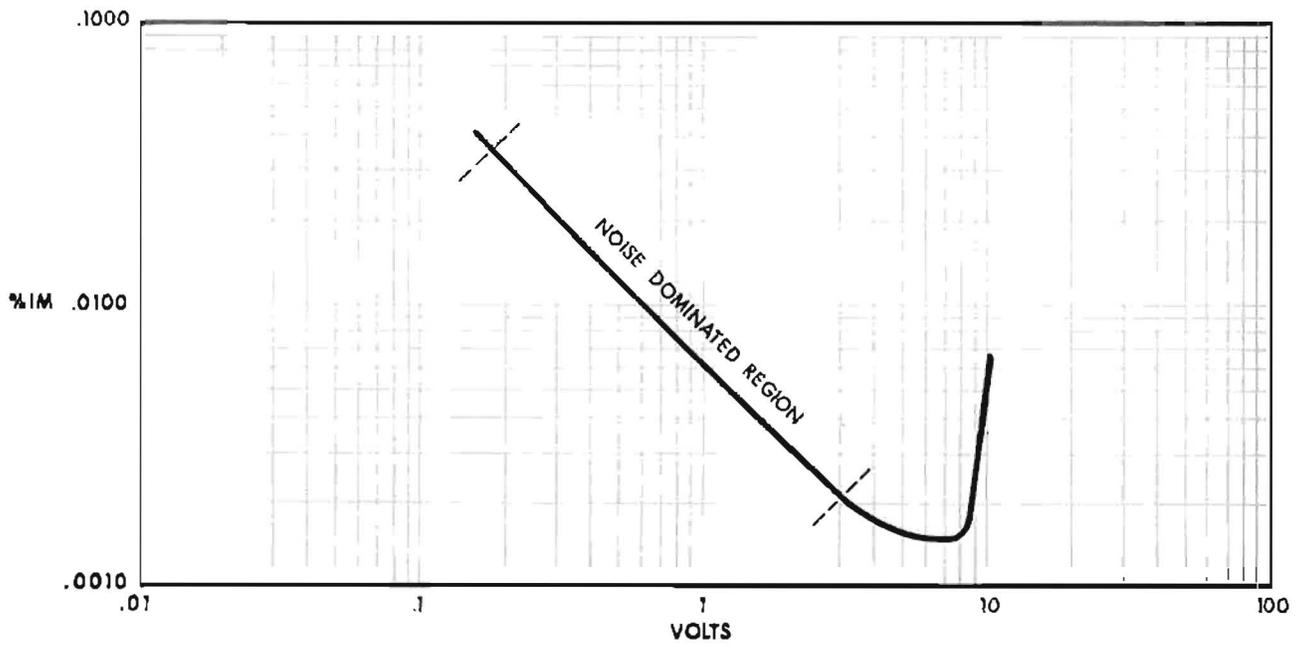
Fig. 2.7 % IM Distortion: All Controls Flat with IHF Load
