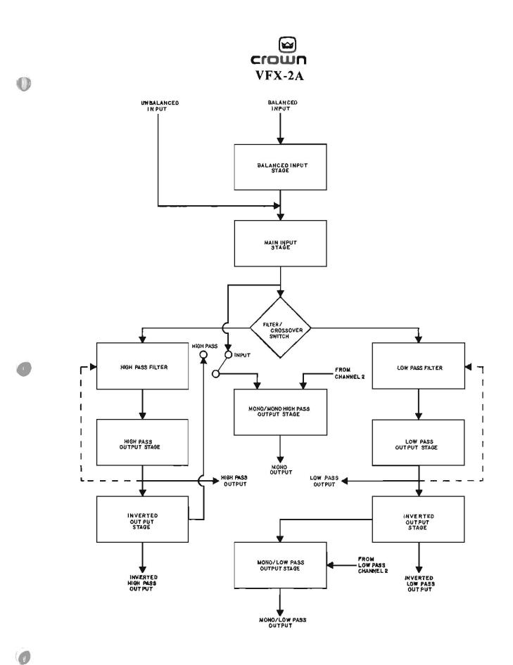
Fig. 4.2 VFX-2A Block Diagram
