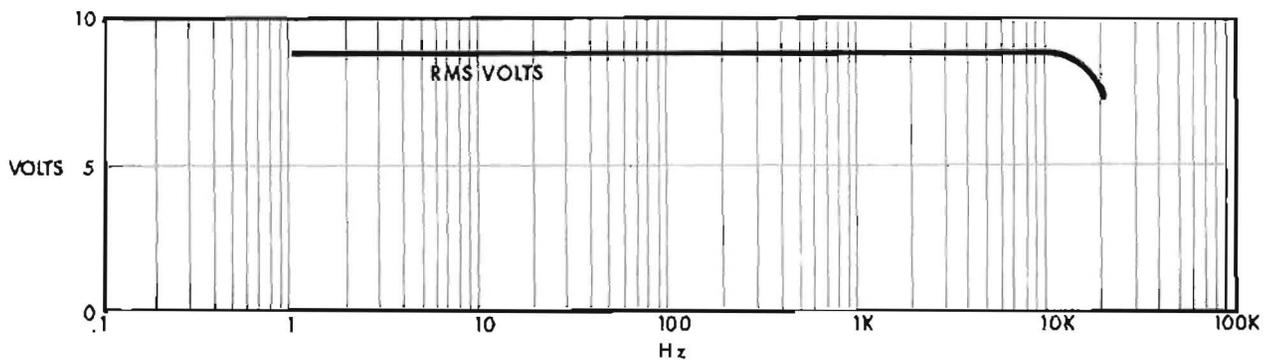
Fig. 2.5 Typical Maximum Output: IHF Load
