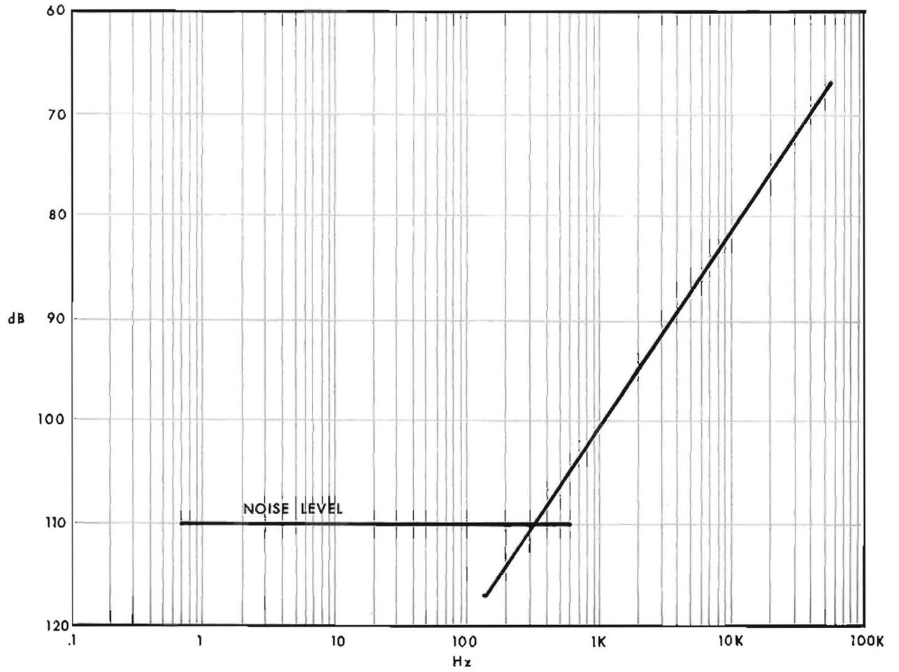
*Fig. 2.6 Typical Common Mode Rejection*
