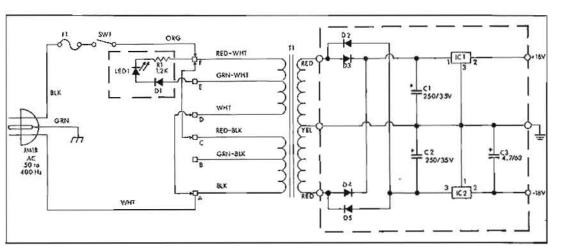
POWER SUPPLY SHOWN WIRED FOR 120 VAC. FOR OPERATION AT ANOTHER LINE VOLTAGE, FOLLOW CONVERSION CHART BELOW. SELECT. THE CORRECT VOLTAGE: CAREFULLY IDENTIFY ALL WIRES & FORE PROCEEDING. THE SIX TRANSFORMER PRIMARY WIRES ARE SOLDERED TO AN ADJACENT TERMINAL STRIP. (A, B, C, D, E, and F). ONLY FOUR WIRES ARE USED IN ANY CONFIGURATION.
