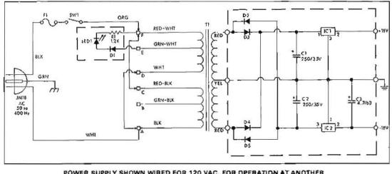
POWER SUPPLY SHOWN WIRED FOR 120 VAC. FOR OPERATION AT ANOTHER LINE VOLTAGE, FOLLOW CONVERSION CHART BELOW. SELECT. THE CORRECT VOLTAGE; CAREFULLY IDENTIFY ALL WIRES BEFORE PROCEEDING. THE SIX TRANSFORMER PRIMARY WIRES ARE SOLDERED TO AN ADJACENT TERMINAL STRIP, (A, B, C, D, E, and F). ONLY FOUR WIRES ARE USED IN ANY CONFIGURATION.
