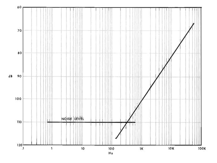
Fig. 2.6 Typical Common Mode Rejection
