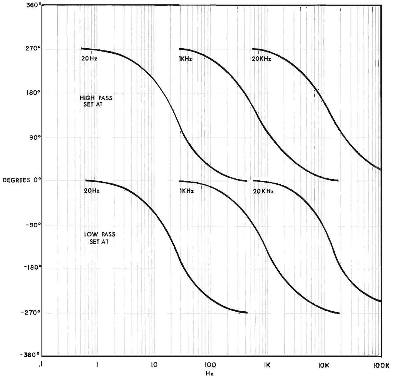
*Fig. 2.3 Typical Phase Response: High and Low Filters*
