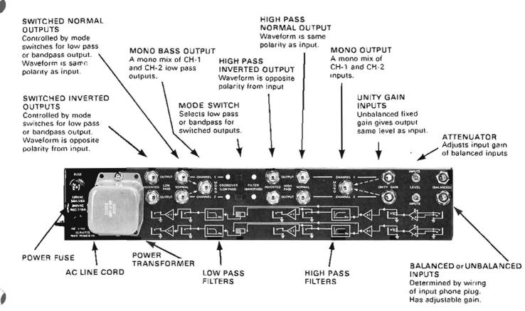
Fig. 3.6 Rear Panel Controls and Connectors
