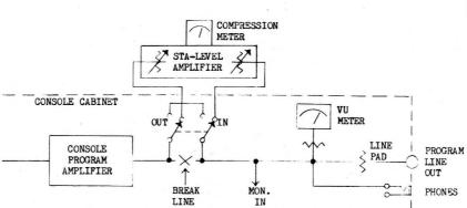
Almost any console is easily modified for use with Gates' STA-LEVEL Amplifier as shown above. Simply remove the output from the console program amplifier, as shown by the break, and connect to the input terminals of the STA-LEVEL Amplifier. Connect the output of the STA-LEVEL Amplifier to the output circuit of the console. The use of a console utility switch, or an external switch, will allow the STA-LEVEL Amplifier to be switched in or out of the circuit as desired.
