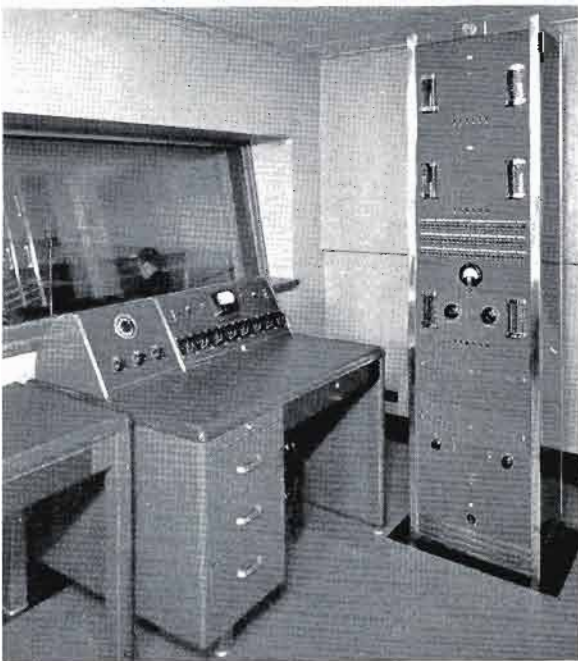
A Studio Control Console and Rack built for WFBR, Baltimore, Md.
