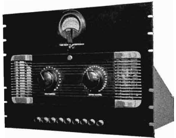
Typical RCA DeLuxe Front Panel, Chromium Lowers Enhance Appearance and Provide Additional Ventilation
