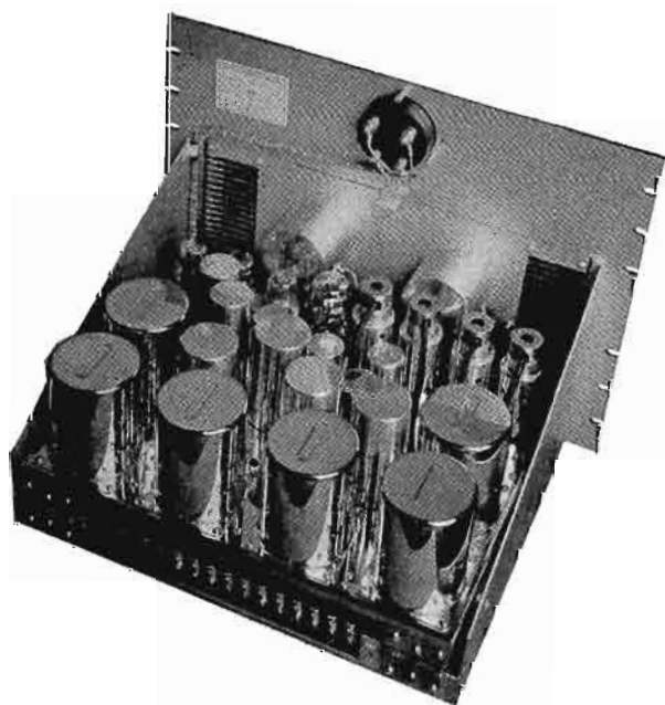
Rear View of 40-D. Substantial Hinges Allow Quick Chassis Opening for Inspection
