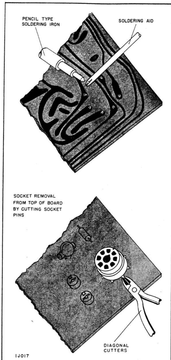
Figure 9. Removal of Multi-Element Component
