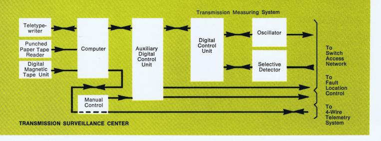
remotely operated switched access network provides the necessary connections to perform the measurements.
