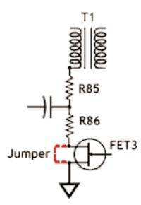
This block diagram is also on Page 227 (Figure 24) in the VRC2000 Installation and Operations Manual. This block diagram is also on Page 84 (Figure 24) in the VRC2000 Installation and Operations Manual (Rev. 2.00). Typical readings of the DTMF level: U16, pin 8 < 1 Vpp when receiving the DTMF tone. If more attenuation is needed even after the modification has been done to FET3, R49 can be changed from a 20kOhm resistor to a 39kOhm resistor.
