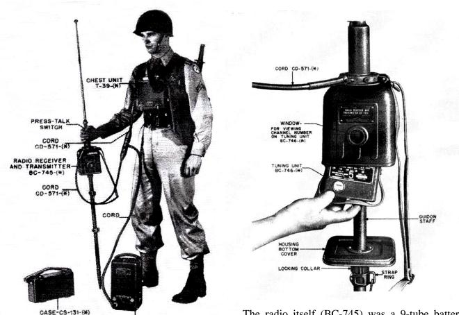
The radio itself (BC-745) was a 9-tube battery filament low HF single-channel, voice only AM, fixed-tuned unit that was little more than an
