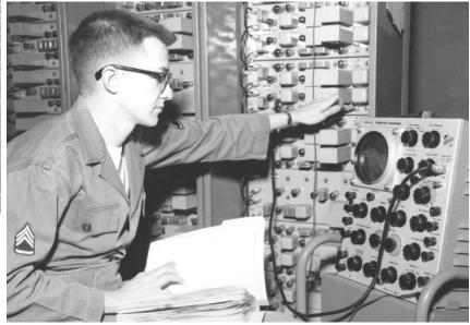
AN/FRC-23 by the Chief Signal Office. The total vacuum tube complement is about 360. Mean time between failures (MTBF) is long and due to tube failure. Average of all 8235<sup>th</sup> microwave station terminal failures was about one every 8 months.
