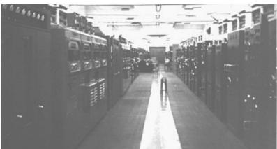
panel open at right showing 120 potentiometers at top and servo amplifiers at middle of rack.
