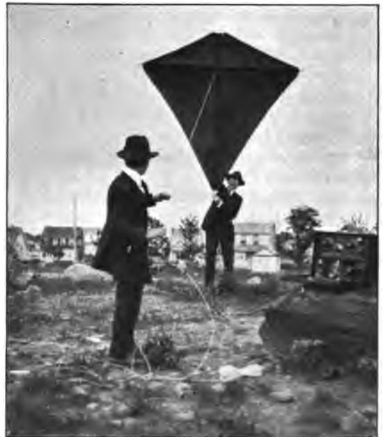
Ashore, the kite-supported antenna materially increases the distance over which radio broadcasting may be received. The kite in this illustration is 7 ft. high
