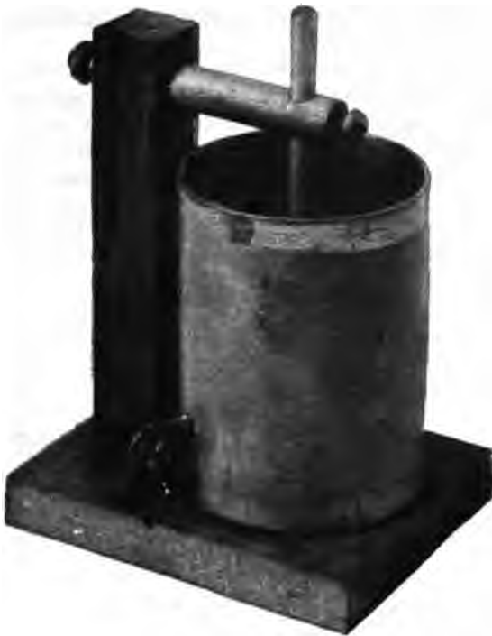
FIG. 9 Electrolytic rectifier suitable for charging 20 to 60 volt B battery from alternating current
