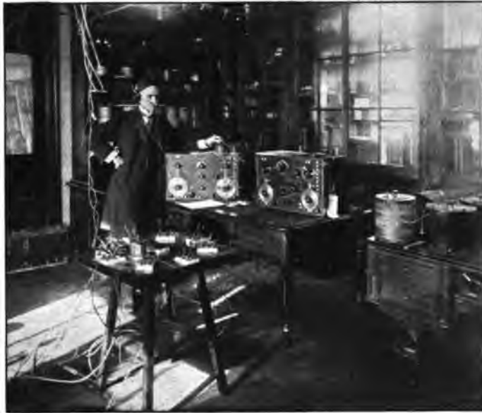
Dr. Rogers using an underground loop antenna receiving a radio concert 220 miles. On the table in the foreground a group of switches, connected to various underground antennas, serve to alter the direction of reception and the wave length
