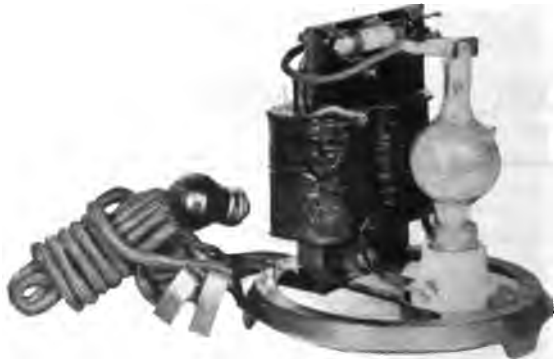
FIG. 16 Gas tube rectifier with cover removed
