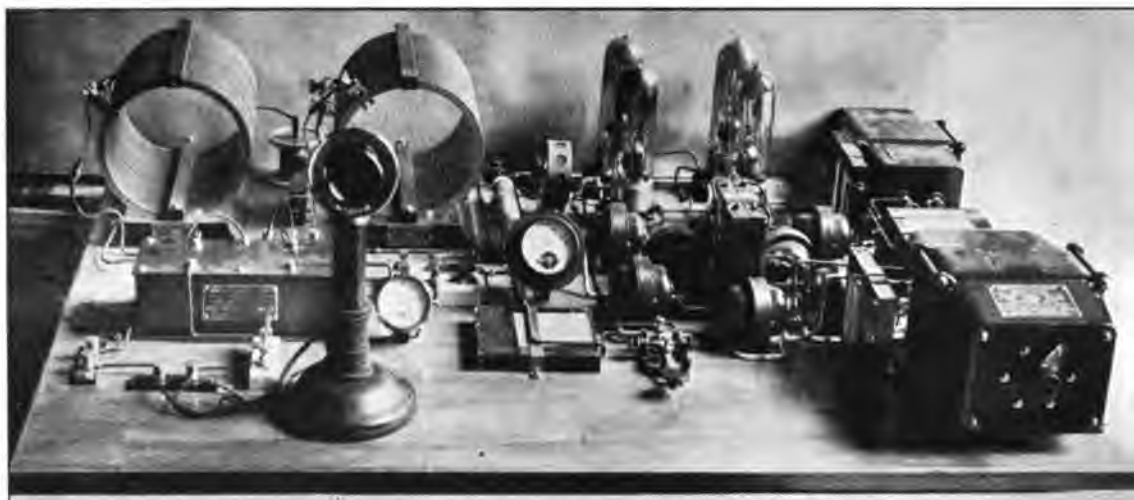
This is a highly refined vacuum tube transmitter circuit, such as is used for instructional and experimental purposes in colleges and laboratories. Completely wired, as this set is, it would be a valuable asset for any dealer, helping him to sell units
