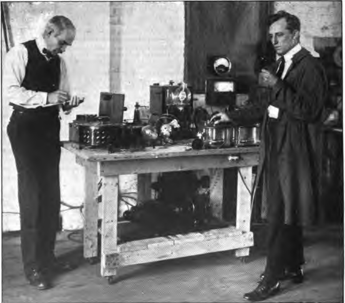
Dr. De Forest measuring the current in various circuits employing a large sized vacuum tube for wireless telephone transmitting
