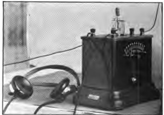
A new compact receiving set, the Federal, Jr., of the Federal Telephone & Telegraph Company
