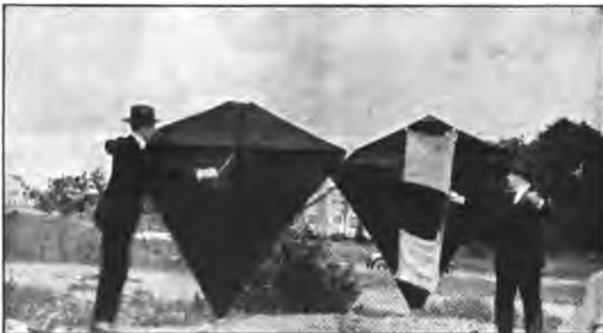
Here are two types of kites employed by the author in experimenting with the portable receiver. For all around use the left hand one is more suitable, but the right hand kite is better for an extremely high wind
