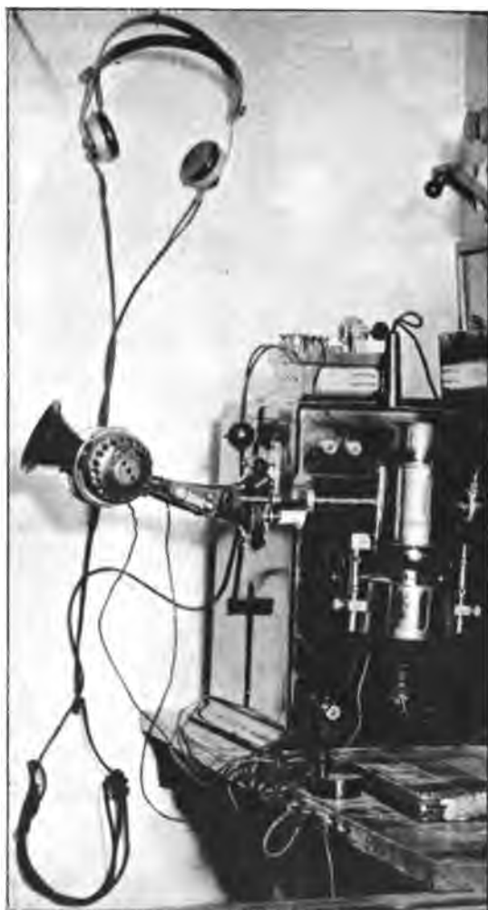
De Forest radiophone installed in Metropolitan Tower for New York to Paris tests. This transmitter was of the arc type and the arc chamber may be seen to the right. Parallel microphones were employed to modulate the antenna current
