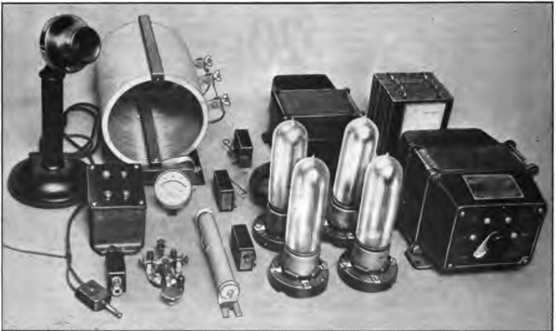
All the necessary parts for a complete 100 watt wireless telephone or telegraph transmitter are shown in this picture
