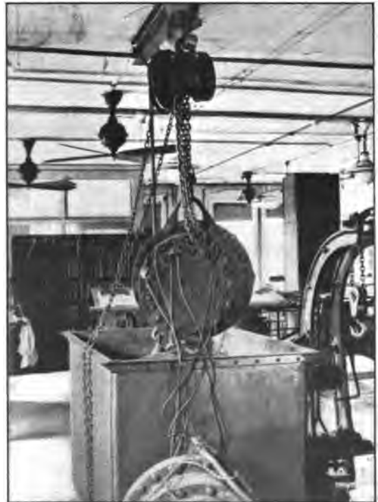
C. Oscillator used on submarines for telegraphing under water, and for telephoning between submarines submerged to a depth of 100 feet at a distance apart of 10 miles
