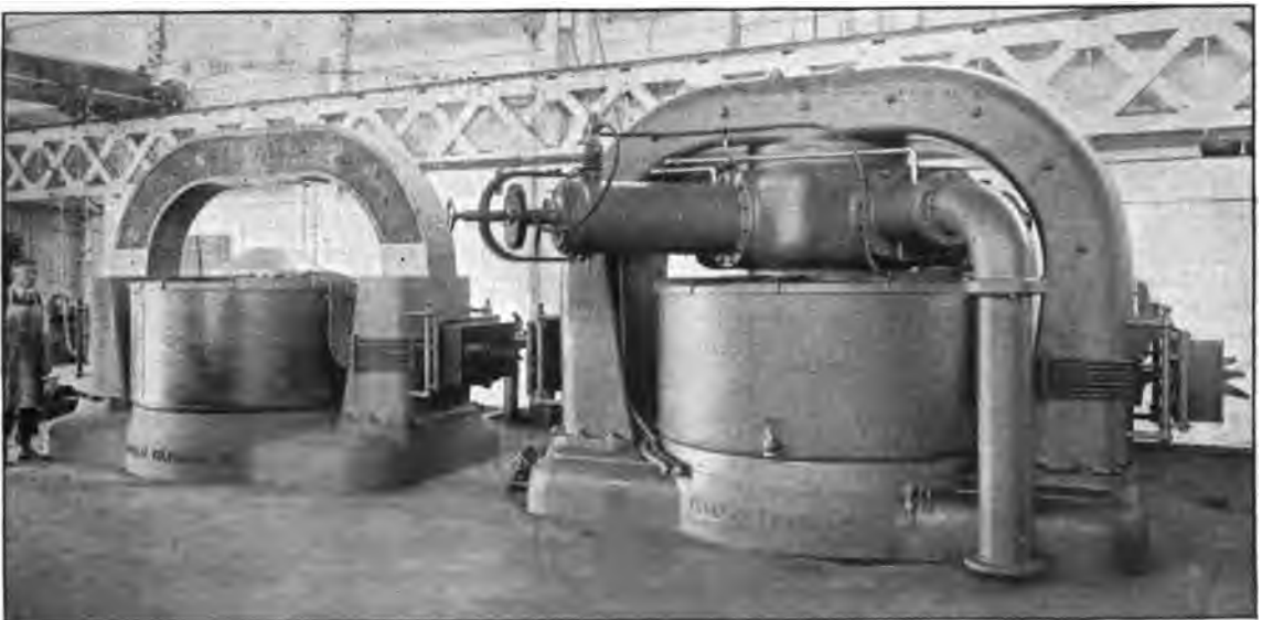
View of the Cavite and Pearl Harbor arc converters under manufacture and assembly at the Federal Telegraph Company's factory at Palo Alto, California
