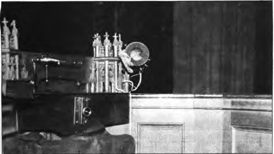
The microphone in the pulpit of Calvary Church, Pittsburgh, Pa. Note its location and the felt padding used to guard it against vibration
