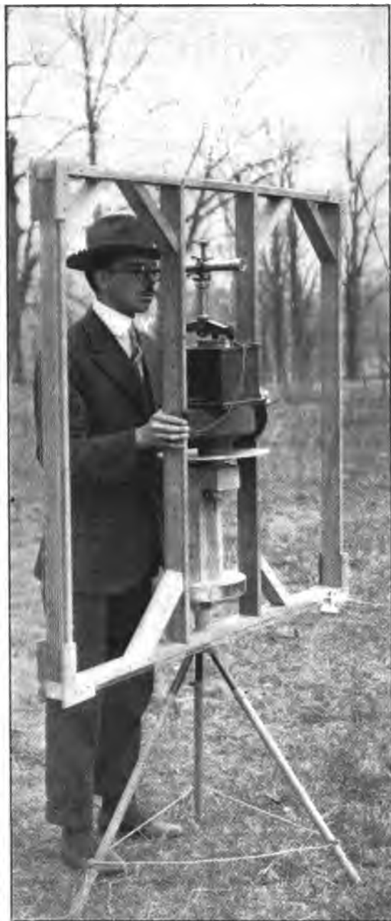
Radio direction finder frame on which telescope is mounted for use in sighting on the radio transmitting station. The scale of degrees is the circular disk just below the hand of the observer
