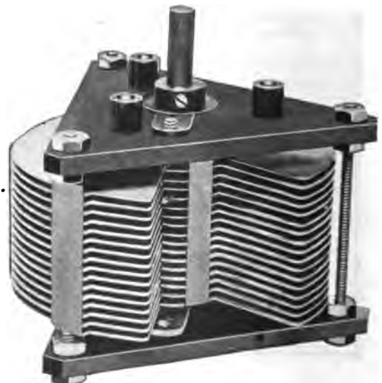
New variable air condenser of the General Radio Company, Cambridge, Mass.
