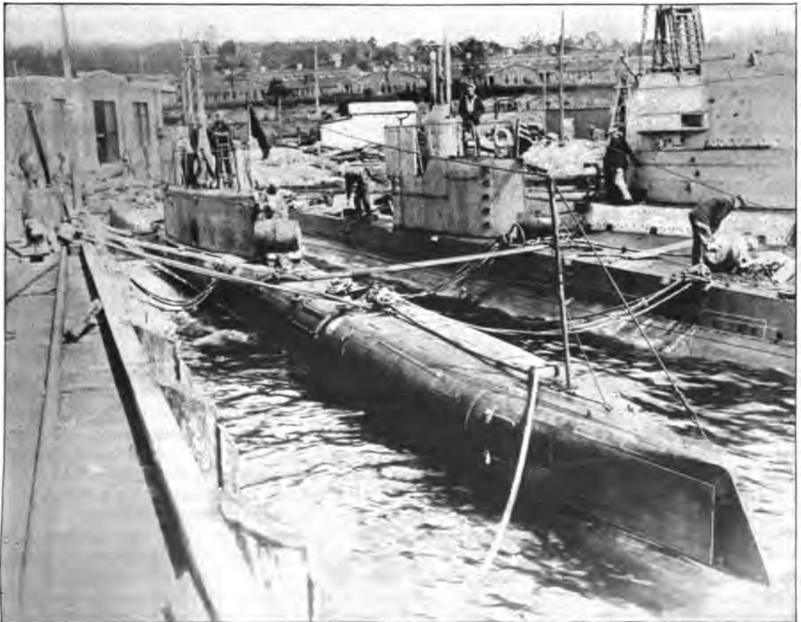
Submarine equipped by the Bureau of Standards, Department of Commerce, with special type of antenna for under-water radio reception and transmission
