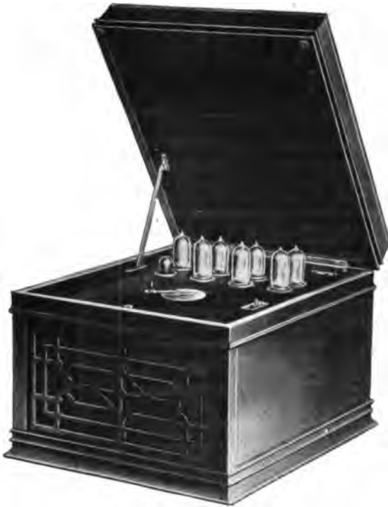
Aeriola Grand showing the vacuum tubes and ballast tubes in place, the switch which controls the entire current supply, and the single control lever used to tune in desired and tune out undesired broadcasting stations
