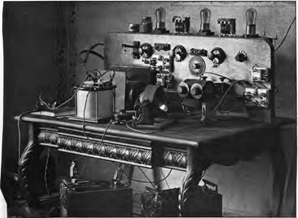
This Radio Regenerative Receiving Set, built by A. C. Philips, Hempstead, N. Y., has proved very effective. The antenna is composed of four strands of solid copper wire spaced two feet, eighty feet long, with a twenty-one foot lead-in. Height 51 feet. A home-made inductance wound on cardboard is used, with movable secondary, and taps on primary. A home-made variometer is used in the circuit as a tickler. The detector and two step amplification is made of standard parts. Double pole double throw switches connect to honey comb coils for long wave lengths. The following stations have been regularly and plainly heard. WJZ—WGI—WBZ—WGY—WWZ—KDKA—WDL—NOF—2XJ—IBKA—WYEB. The layout was arranged after a great deal of experimenting with different makes of standard parts, and left as shown owing to the fact that results were most satisfactory. Six sets of phones connected in series around the receiving room afford convenience and comfort to those who listen in.
