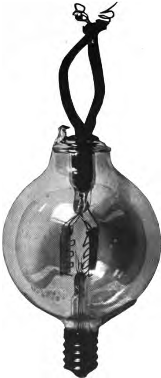
© Paul Thompson This is a real old De Forest audion. Several years ago radio amateurs saved for long periods to procure one of these magic bulbs. As may be observed, two filaments, two plates, and two grids were employed. The stability of this type tube was anything but constant due to imperfect evacuation
