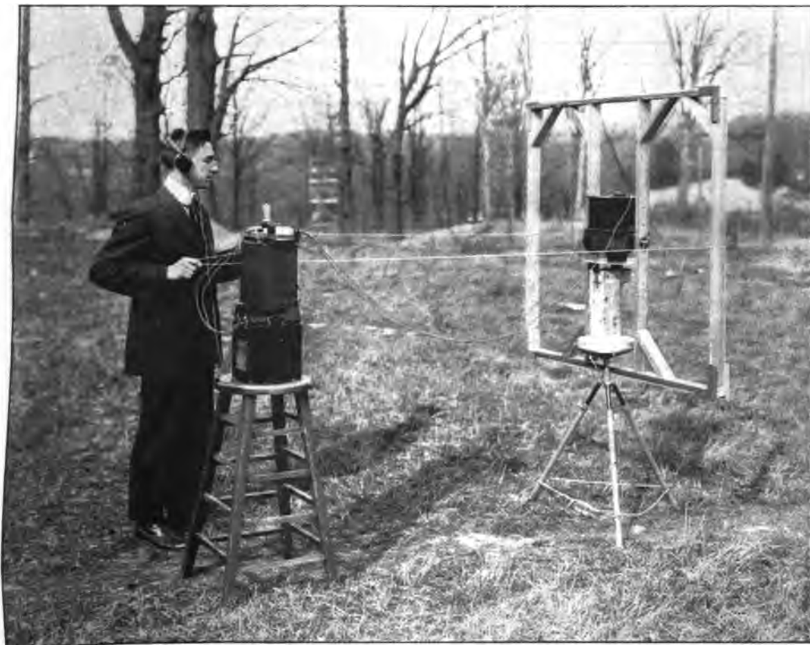
Radio direction finder in use in obtaining exact position of passing radio waves. The observer turns the frame by means of cords in order to be sure that his body has no effect on the direction of the waves. The detector and batteries are seen on the stool near the operator
