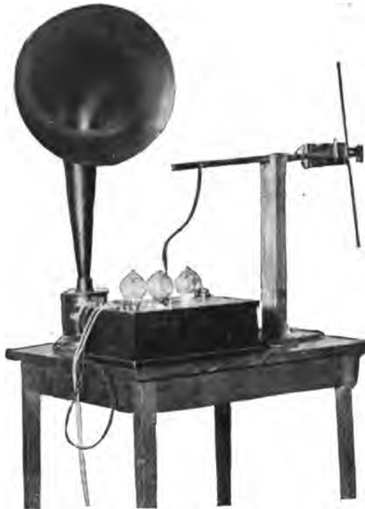
The receiving outfit used by Marconi to demonstrate the reception of extremely short waves sent out by a directive antenna. For the demonstration, he used a loud speaker of American make so that the audience could observe the effect of his directional antenna. The signals of extremely short waves are picked up and then pass through a circuit similar to the superheterodyne and thus changed to a wavelength of six hundred meters. Although six hundred meters is the wavelength for ship use no interference is experienced from this source because only those waves which influence the detector circuit are passed on. This feature of the receiver was not pointed out by Marconi and is therefore not generally realized
