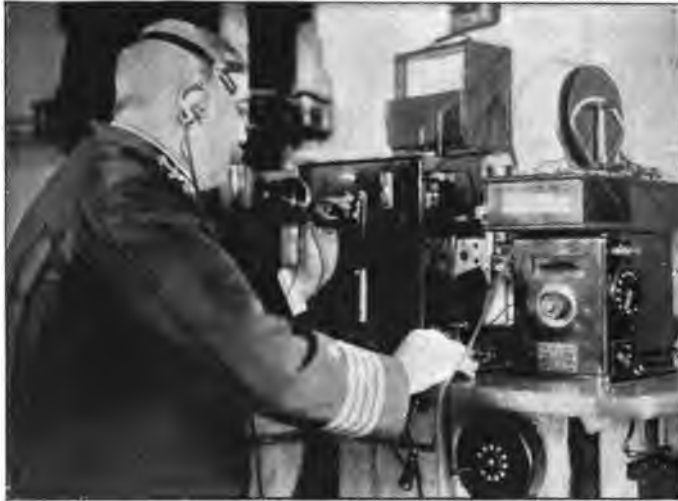
Capt. Ingersoll, Chief of Staff to Admiral Evans using a radiophone on the U. S. S. Connecticut at Hampton Roads in 1907. In the upper right hand corner of the picture may be seen what was termed a pancake receiving oscillation transformer, the number of turns on either coil being regulated by the movement of a slider arm
