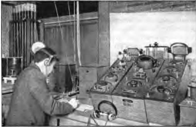
In 1908 messages were sent from the Metropolitan Tower, New York, to Milwaukee and Key West by the "Sparkless" radio telegraph. The arc chamber employed for this transmission may be seen at the extreme left over the operator's shoulder. The huge boxes before the operator constitute the receiving equipment. The radio amateur of yesteryear will recognize the old fashioned variometers, variable condensers, audion detectors, and adjustable pillar inductances
