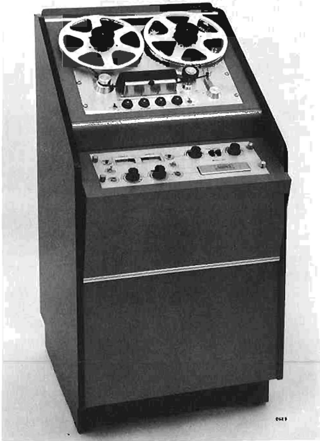
A console mounted Ampex Model 354, two channel recorder/reproducer
