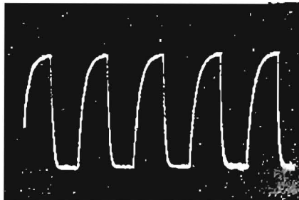
FIG 5 UNMODULATED 24 VOLT IF (P-P) 900 KHZ SIGNAL AT COLLECTOR OF Q-4 ON PLUG-IN CARD A-3
