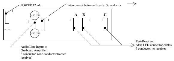
CIRCUIT BOARD FBAFC3A: holds the AUDIO SELECT 4 position switch, TEST/RESET switch, ALERT LED's and associated circuitry.
