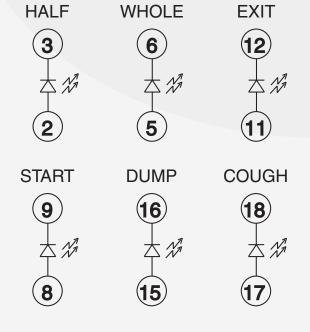
Note: The numbers within the circles refer to pins on the 6000's rear panel DB-25 connector which is labelled REMOTE CONTROL & INDICATORS.
