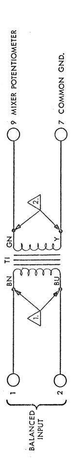
SPARTA 23W7, 10K ohms, 1:1 TURNS RATIO. OPTIONAL, 600 ohms, 1:1 TURNS RATIO.
