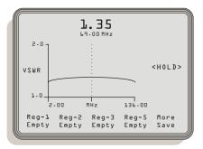
The desired units, band, and scale should be selected. You should be in the single hold mode and the trace you want stored should be displayed. If continuous sweep type is selected, the trace displayed when you save will be stored.
