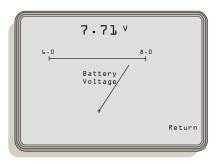
If the voltage measured is less than 7V you should charge the batteries.
