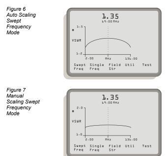
In the single frequency mode Auto Scaling sets the measurement unit scale so the pointer is mid range of the previous reading. The maximum and minimum scale values are approximately 10% higher or lower than the measured value.
