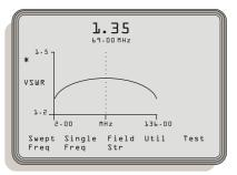
Single Frequency mode displays the unit of measure in a simulated analog meter graphic. This mode, particularly when audio is on, is useful when tuning an antenna.
