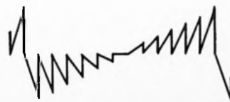
Detail D. Simulated velocity error signal generated by velocity compensator
