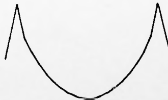
Detail E. Output of velocity compensator ( D + B )
