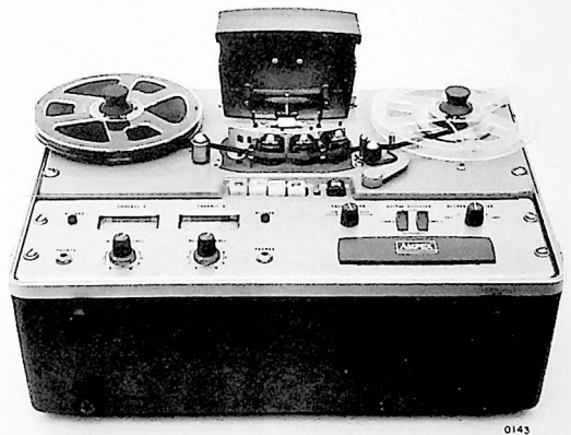
Typical professional quality recorder/reproducer in portable case. Ampex Model PR-10-2 fits either a portable carrying case or will mount without modification in a normal 19-inch rack.
