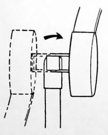
NOTE Each radial beam is located 180° across hub from beam on opposite side.
