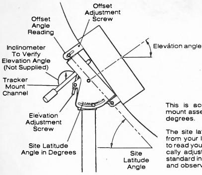
This is accomplished by inclining the polar mount assembly to read directly in site latitude degrees.
