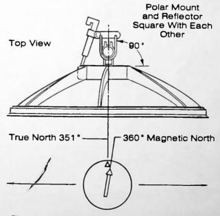
The above illustration uses a magnetic variation of  $(-9^{\circ})$  resulting in a true north reading of 351° as would be the case in Oklahoma City, since it is located on the  $(-9^{\circ})$  variation line.
