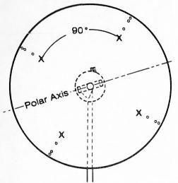
Fourth inboard hole remove 5/8 screw & replace with strut (large end) and 3/4 screw
