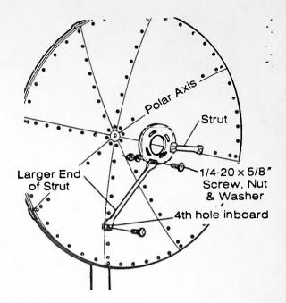
Secure feed mount plate under strut flanges with  $1/4-20 \times 5/8^{\prime\prime}$  long screws, nut and washer as illustrated. Rotate reflector to opposite side and attach final two struts.
