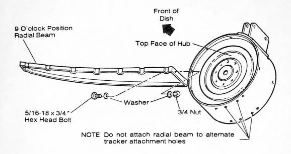
Continue installing three additional radial beams in a counterclockwise direction. Then rotate hub up and over polar mount to the opposite side and install the remaining four radial beams in the same manner.
