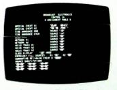
Assignment Table Display Initial system assignments are easily made from the keyboard while viewing this display. Unlike most other sytems, Control 16's source assignments for Time Announce, Back Time/Dead Roll, Voice Track, etc., are done in software for easy changing should the need arise.
