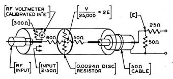
Figure 6. RF Attenuator and Voltmeter
