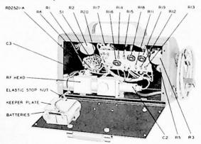
Figure 11. Interior View—Component Layout, Including Mounting Of Batteries.
