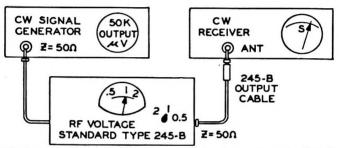
RF voltage at high level is obtained from the signal generator and adjusted to give the desired output. The attenuated output is picked up on a receiver and a reference reading noted. Calibration is in terms of open circuit voltage at the end of the output cable.
