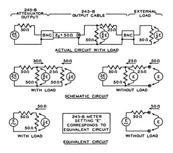
Figure 4. Derivation Of Equivalent Circuit Of RF Voltage Standard Output System Assuming A Matched Load. impedance of the receiver. This yields 0.5  $\mu$ v across the receiver input terminals.
