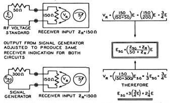
Figure 8. Signal Generator Output Determination When All Three Impedances Are Different.
