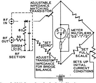
Figure 9. RF Voltage Standard—Basic Circuit.
