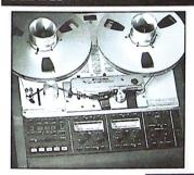
The **Studer A807** was conceived as a multipurpose tool for recording studios and broadcasters. The A807 has a highly perfected tape transport design with advanced drive technology features: two rugged direct drive AC spooling motors, brushless DC capstan motor, comprehensive function selection and digitally controlled analog technology.
