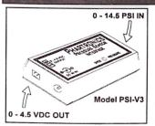
The Phartronics Pressure Sensor Interface provides a very precise sample voltage of 0 to 4.5VDC that varies linearly with line pressure. The DC sample is compatible with any brand of remote control. To set a Lower-Limit alarm on the pressure sample input of your remote control simply "T" into your existing pressure line to provide a line pressure sample and connect the output sample voltage to your remote control.
