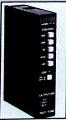
**Fostex TT-15** is a 9V battery operated, 5-frequency sine wave oscillator (40 Hz, 400 Hz, 1, 10 and 15 kHz) with 3 selectable output levels (-30, -10 and 0 dB), is useful for spot checking frequency response, calibrating mixers with tape recorders and other level matching jobs.
