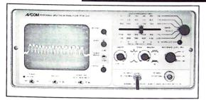
The Avcom PSA-35A is a portable spectrum analyzer with LCD frequency counter readout. It accurately measures wide band signals used in the TVRO industry. Frequency coverage from 10MHz to over 1750MHz, and from 3.7 to 4.2GHz. Please specify voltage.
