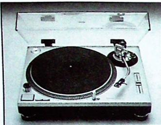
The **Technics SL-1200MKII** is a quartz-locked direct drive turntable that is virtually feedback-proof because of its special base design. The platter is damped on both sides to avoid ringing. Its high starting torque brings the platter to rated speed within 0.7 second. Includes base, tonearm and dust cover.
