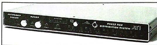
The **ATI PB2X8 Press Box** Distribution System has two balanced mic/line inputs with switched phantom power and low cut filter on mics. Both inputs have individual gain controls and are switchable together or separately into any of eight transformer balanced adjustable outputs. Calibrated test tone oscillator • Switchable LED display • Line level XLR connectors in and out • plus 1/4" and 3.5mm phone jack outputs at -10dBu.
