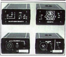
A test instrument for the audio installer or soundman which indicates absolute polarity of most audio devices or may be used as a cable tester. The send unit has balanced 1/4" and XLR jacks, an unbalanced 1/4" speaker out jack and an internal speaker. The receive unit has 1/4" and XLR jacks, a sensitivity control and an internal microphone. Both units are housed in high impact padded ABS cases and are powered by a 9 volt battery.
