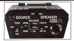
This Whirlwind Cable Tester can test cables with any combination of XLR. 1/4" or RCA phono plugs for shorts, opens and phase. The handsfree design allows manipulation of cable to locate intermittence. An on/off switch is provided, with LED to indicate sufficient test-
