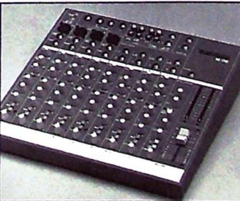
The **Tascam M08** compact mixing system features: 12-Input (4 mono, 4 stereo) • 4 XLR inputs • 2-Band EQ on all channels • 2 Dedicated AUX sends (pre and post) • 4 Mono effects returns • Mute and PFL on each input channel • Dedicated 2-track input • and 60mm Linear master fader.
