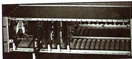
**STL PLUS Basic Package (4200)** includes two TDM-163(115) T1 multiplexers, one uncompressed stereo audio transmitter module, and one uncompressed stereo audio receiver module, with module adapter.
