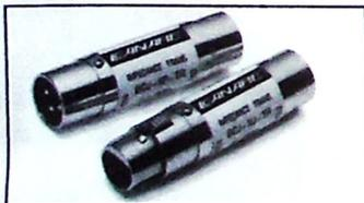
**Canare Impedance Transformers** allow 75Ω coaxial transmission of all 2 channel AES/EBU Digital Audio signals. Low cost and easy to use, the I/O adapters, are designed to passively convert all standard AES/EBU digital audio signals from 110Ω/XLR3 Output (@ 4.5 Volts), to a 75Ω BNC coaxial cable and then back again to a 110Ω/XLR3 Input (200mV min). Also provides excellent rejection against hum and noise.
