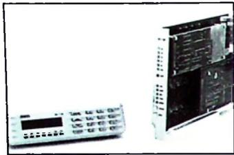
Adtran's **ISU128** is a stand-alone ISDN Service Unit that connects data terminal equipment directly to the ISDN network. The ISU128 includes NT1 network termination and terminal adapter functionality. Synchronous and asynchronous rates are supported through a V.35 or RS-530 interface. For speeds over 64 kbps, the industry standard BONDING protocol is used to aggregate the two 64 kbps "B" channels.
