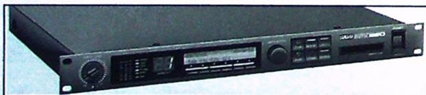
The **Yamaha SPX-990** has a wide selection of professional quality digital effects. It has 80 preset effects and 100 memory locations. True stereo (2-in/2-out) configuration allows stereo sources to be processed without disrupting the original stereo image. Effects include: reverb, early reflections, delay & echo, modulation, pitch change, pan, freeze, and complex effects. Inputs and outputs are analog, electronically balanced, with XLR and TRS 1/4" connectors. A/D-D/A are 20 bits. 1U
