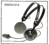
The Sennheiser HMD410-6 is a supraural, open-aire,  $600\Omega$  headphone (20-18kHz) with a dynamic supercardioid,  $200\Omega$  boom mic (50-12kHz). Comes supplied with a 6' stranded steel cable terminated in stripped and tinned leads. Weight 18 oz.
