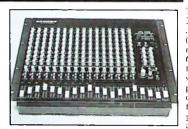
The Samson MPL 2242 is a 22-channel, 4-buss, rack mountable mixer. It has 22 total inputs, (10 XLR balanced featuring a lownoise, padless preamp design, and 6 1/4" TRS stereo inputs). Other features include: 4-band EQ • 4 stereo aux returns • 6 aux sends, (1 pre-and 5 post-fader) • 4-bus design (using 4 dedicated group faders for submixing) with discrete group and main summing outputs • and more.
