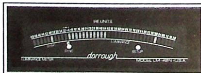
The **Dorrough Video Luminance Meter Model 40-N** is an NTSC video level meter that displays the video signals of average and peak luminance, sync level, and setup violations. Sync range -50 to -32 IRE. Meter resolution 4 IRE per LED.
