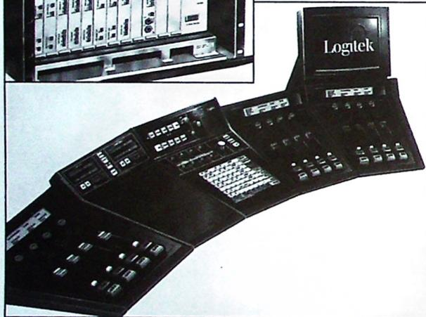
**Logitek's Serial Sound System** consists of a 12-slot mainframe which can hold up to eight, 8x8 mono/4x4 stereo analog or digital I/O cards, two DSP audio processor cards, two communications processor cards and up to two power supplies. The mic pre-amp unit is housed externally and offers four independent pre-amps with balanced I/O on XLR connectors.
