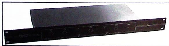
The **Zercom Telephone Hybrid** provides full duplex audio. Zercom's Telephone Hybrid nulling circuit has two null controls and active balanced inputs and outputs with adjustable gain. The telephone line, tip, and ring connection is user selectable on the rear panel for a direct DC line hold or capacitor isolated to prevent DC flow through the hybrid's telephone line transformer.
