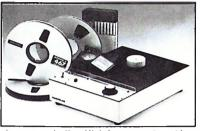
AUDIOLAB TD-4A • Erases audio, video and data tapes; U-Matic cassettes up to 750 oersteds and reels up to 16 inches in diameter and 1 inch in width. • Provides a 2550 effective Gauss Field in HI mode • Built in timer has adjustable "ON" cycle and automatic shut-off • Automatic cooling fan operation • Overheat light with automatic thermal protection prevents exceeding duty cycle on HI position • Thermal protection resets to normal opera-
