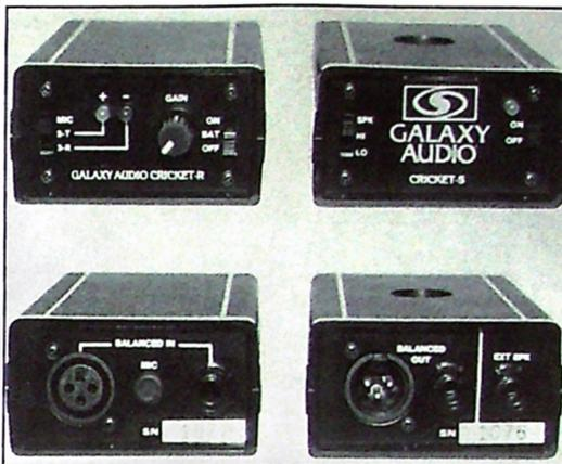
A test instrument for the audio installer or soundman which indicates absolute polarity of most audio devices or may be used as a cable tester. The send unit has balanced 1/4" and XLR jacks, an unbalanced 1/4" speaker out jack and an internal speaker. The receive unit has 1/4" and XLR jacks, a sensitivity control and an internal microphone. Both units are housed in high impact padded ABS cases and are powered by a 9 volt battery.
