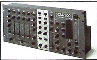
The Biamp SCM7600 is a complete stereo control center, designed to be the heart of a high quality club sound system, with two stereo phono inputs, eight stereo line inputs, and two mono microphone inputs. It has six independent stereo outputs, plus a subwoofer/mono output and a light send output, for maximum flexibility. Biamp has a five year warranty and is made in the U.S.A. 5RU
