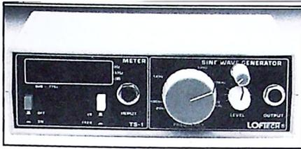
**Goldline TS-1** is three audio test instruments in one unit. It includes: a low distortion audio oscillator with a range of 10Hz to 30kHz; a frequency counter with response of 1Hz to 99.99kHz; and a dB meter with range of -50 to 24dB from 20Hz
