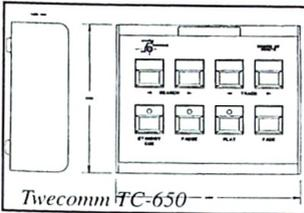
**Twecomm TC-650** is a remote control for the Denon DN-650F, DN-951FA, DN-961FA, DN-980F, DN-990R, and DN-995R CD players and mini disc recorder/player units. The remote has the following functions: Standby-Cue
