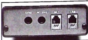
**Gentner's Hybrid Coupler** connects directly to the telephone line and is used to send or receive audio or other information. Its passive design allows you to "tap" the phone line, using the telephone and coupler simultaneously, or it can seize the line. Use it for news or producer feeds, or sending a church service broadcast.
