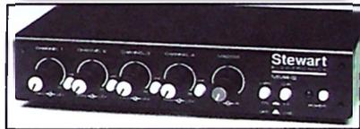
Each of its four balanced mono inputs are individually switchable between microphone and line level, with switchable +48v phantom power. The MM4-S features an individual gain and pan control for each channel, as well as master level control, and switchable balanced output operating levels.
