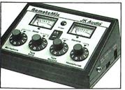
The JK Audio RemoteMix replaces the handset on your analog, digital, PBX, ISDN and single line telephones for professional remote broadcasts. It has balanced XLR and unbalanced RCA line I/O's, one balanced XLR mic input, and an adjustable sidetone null feature. An internal 8Ω, I watt/channel
