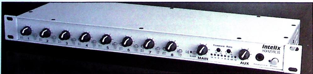
The **Intelix 8002 MCB** is an eight channel, dual buss microphone mixer designed for the broadcast, video field production, sound reinforcement and recording industries. It has: balanced inputs and outputs • 1U chassis • phantom power • level control • LED bargraph • limiter • front panel headphone output • dual busses • and can be AC or DC powered.
