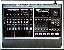
recorder, a digital mixer and studio-quality multieffects (an add-on board option) in a completely self contained unit. Every operation is performed within the digital domain. It has 4 analog I/Os and 2 SPDIF digital I/Os. You can record 4 tracks at once with 8 layers per track making the total number of tracks per song 64. Editing functions include: copy, move,
