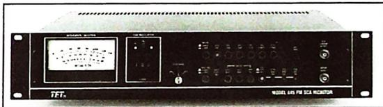
The TFT 845 is an FM SCA monitor with up to three front panel selectable subcarrier frequencies. The 845 can be used to make SCA proof measurements and with one or two optional service channel boards it can provide uninterrupted SCA program or data output(s) separate from the monitor portion. It includes a loss of modulation alarm and a built in modulation calibrator. The 845 has a one year manufacturers warranty.
