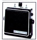
The ATI Audible Noise Generator NG-1 has selectable and adjustable pink or white noise, pulsed or continuous with built-in speaker and an output jack for an external amplifier and speaker. It's battery operated for portable use and includes a wall mount AC power supply for continuous operation.
