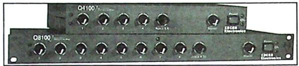
The **Eddor Q4100 & Q8100** microphone mixers have 4 or 8 balanced XLR female microphone inputs with phantom power. There are also 2 RCA auxiliary inputs with a single volume control bringing the units to 6 or 10 channel mixers. Each microphone input has individual volume control. Outputs are balanced XLR male connectors with 600Ω line level and the auxiliary level output is unbalanced RCA type connectors with maximum output of 8 VRMS into 10,000 Ω's.
