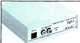
The **JK Audio Tap-1** telephone audio + power interface, separates voice into transmit and receive signals for recording or service simulation. It powers telephone with -48VDC, and provides a 2-wire to 4-wire hybrid.
