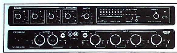
The **Shure FP410** is a portable mixer that automatically keeps unused mics turned down and will only allow one mic to be activated for each source. When someone speaks the Noise Adaptive Threshold activates within 4 milliseconds for speech, not room noise. When no one is speaking, the last mic is kept on to assure a consistent background ambience, until a new one is activated. The FP410 can control multiple wireless mics, work in the effects loop of a multi-channel con-
