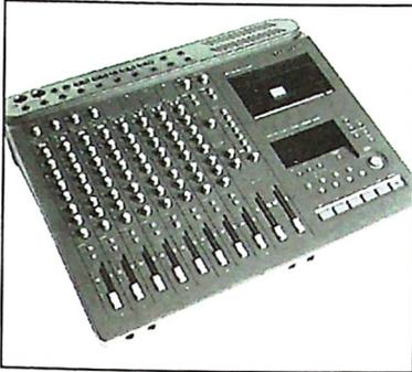
The **Tascam 488MKII Portastudio** gives you the functionality of a professional studio like: 8-track recorder with 8-channel, 12-input mixer • XLR inputs with 48V phantom power • 3 band EQ • auto punch in/out • 2 independent AUX sends • dbx noise reduction • and multi-function, fluorescent meter display.
