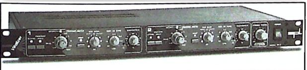
The **SPL Stereo Vitalizer** takes the concept of "audio sweetening" to a new level. Designed to be compatible with the way the human ear perceives sound, the Vitalizer's network of interactive filters actually reshapes the entire audio spectrum so that listeners perceive sounds as louder, clearer and more detailed.
