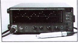
The Audio Control Industrial SA-3050A is an affordable, measurementgrade, one-third octave real-time analyzer designed for audio signal analysis. The SA-3050A offers the following features: 30 one-third octave bandwidth filters • Internal pink noise source • 9 x 30 large-format LED display with 1dB resolution • Six internal memories with battery backup • Averaging for 6 stored response curves.
