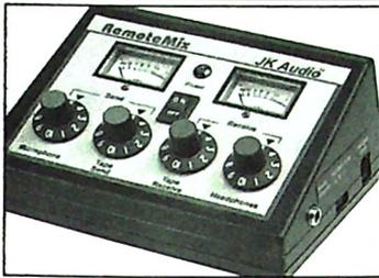
The JK Audio **RemoteMix** replaces the handset on your analog, digital, PBX, ISDN and single line telephones for professional remote broadcasts. It has balanced XLR and unbalanced RCA line I/O's, one balanced XLR mic input, and an adjustable sidetone null feature. An internal 8Ω, 1 watt/channel
