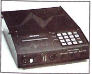
The Comrex Nexus has everything you need for sending great sounding audio over ISDN. Audio codec, terminal adapter and NT1 are integrated into a rugged, 3 pound, easy-touse package. The Nexus provides low delay 15kHz bidirectional audio on 112/128kb/s circuits such as BRI ISDN. It also provides standard G.722 7.5kHz audio at transmission rates of 56/64kb/s. Audio input
