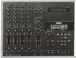
The **Yamaha MT4X** is a 4-track multitrack recorder with flexible mixing facilities and advanced creative control. Each of the four input channels can accept mic or line level signals.
