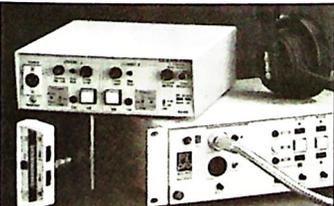
**PL-Pro Party Line Intercom** is designed specifically for the demanding world of broadcast and video production, including multiple built-in IFBs, intuitive front panel controls with big, easy-to-use buttons and bright illuminated call signaling. All stations
