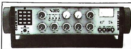
The AEQ MP-10 portable mixer is ideal for remote transmission. It has transformer balanced selectable mic/line inputs, transformer balanced
