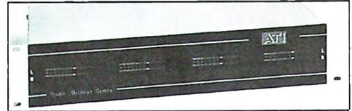
**ATI Nanoamp Series Metering** has balanced bridging inputs, each drive ten segment, multi-color LED bargraph meter display. 0 dB internally selectable @ -10, +4, +8 dBu. Front panel trimmers allow for precise calibration at 0VU.
