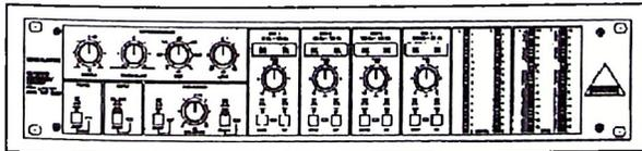
**Microcon Systems Banshee IV** is a stand-alone, 2 RU analog processor incorporating a 4-band leveler, compressor, peak limiter, intelligent peak clipper and stereo generator with an internal composite clipper working in concert to produce a loud, clean, almost tube-like processed sound. Just give us a call to arrange an evaluation!
