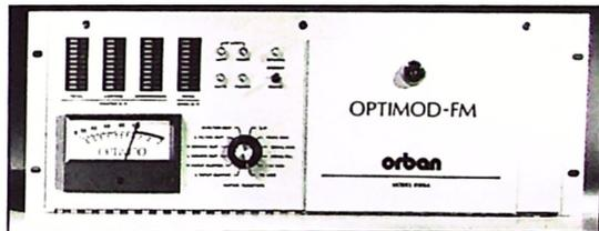
**Optimod-FM 8200ST** is installed before your STL at the transmitter to protect it from peak and high frequency overload. The 8200ST also controls average levels on the link to maximize its dynamic range, translating to improved signal quality at the receiver.
