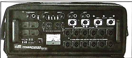
**Whirlwind's PressPower** takes two transformer isolated XLR mic/line inputs and distributes them to sixteen transformer isolated XLR outputs (12 mic/-50dB, 2-line/0dBV, 2-line/variable). A headphone output is provided with a level control, plus, to expedite setup, a 1kHz tone is available. Powered by four 9V batteries or AC (110/230), the PressPower can be rackmounted or used with the included carrying case.
