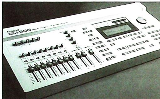
The **Roland DM-800** Multi Track Disc Recorder is a compact, stand alone unit - a completely dedicated digital audio workstation. It performs all digital mixing operations from audio recording editing, track
