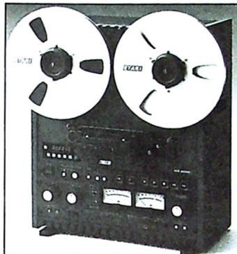
The Otari MX5050 series feature: built in mini-autolocator with three one-touch cue point memories, search zero and repeat functions. The transports are very smooth with micro-processor controlled logic, motion sensing and dynamic braking. Standard features include a 37 pin parallel I/O,  $\pm 20\%$  speed control, transformerless active balanced inputs and out-
