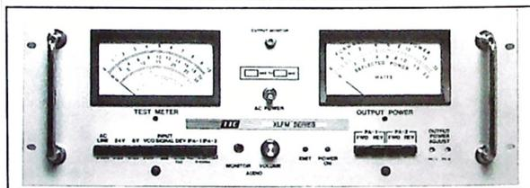
TTC developed the **XL-FM Translators** for customers who needed a way to fill gaps in their coverage. The XL-FM accepts a single FM channel, converts it to another FM channel, and provides for one or two outputs of 10 Watts.
