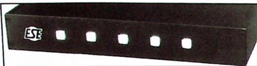
**ESE ES305 News Talent Count-down Display** is mounted to a camera so talent can see the five bright orange lights that extinguish one at a time the way a director counts down. It can display a 5 second count-down or start with 5 seconds of steady lights prior to count-down. The ES305 can be operated from 120VAC 60Hz or 400Hz, or it can run on 12VDC. It comes in a black anodized case measuring 1.6"H x 10"W x 5" D and weighs less than 2 lbs.
