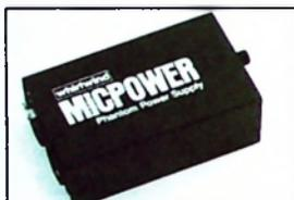
The **Whirlwind MicPower** is a portable phantom power supply for use with most electret condenser mics. It supplies +12 to 18Vdc under nominal loads at the microphone input, and the output of the unit is AC coupled. The unit operates on two 9V batteries, and an LED sensing circuit indicates sufficient battery power.
