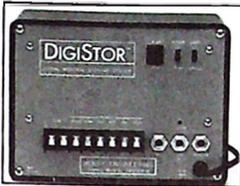
**Henry Digistor** is a digital message storage system that is ideally suited for radio and TV station information lines. The message is stored in digital memory with battery back-up. Digistor can be programmed to play the message only once, or continuously until the caller hangs up. There is no re-cue time; the caller always hears the message from the beginning.
