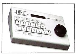
DNF SW1X8 RS422 Switcher allows the ST200, ST100 Universal VTR Controllers, edit controller, or any other RS422 VTR Controller, to control of up to 8 VTRs. At the press of a button, select 1 out of 8 VTRs for individual control, select a group of VTRs to control, or gang roll all 8 VTRS. Connect 2 or more SW1X8 RS422 Switchers to control more than 8 VTRS. The SW1X8 is a highly effective Routing and Distribution system. 1U
