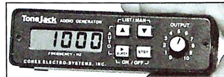
with precise frequencies from 1Hz to 29,999Hz. It is useful in testing the frequency response of systems, filters, tone sensors, etc. It is powered by a 9V battery or external power and has an RS232 interface that allows a computer or terminal to control all the normal front panel functions.
