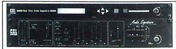
The **CRL Audio Signature** is a digitally-controlled AGC/4-band compressor that is programmable, allowing a fully customized sound to be achieved. The Signature can be remote-controlled via a PC or "day-parted" using the optional CRL real-time Event sequencer. The Audio Signature works well in front of most modern stereo limiters.
