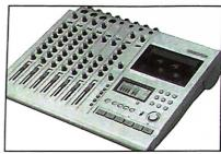
4-track recorder with 12-input mixer (8 mono, 2 stereo) has balanced XLR inputs, sync in/out for use with MIDI, auto locators, auto punch in/out and two effects sends.
