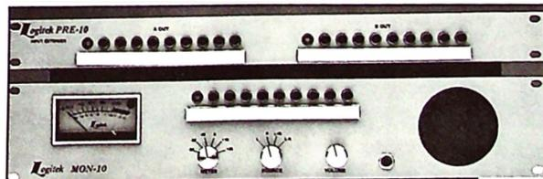
The Logitek PRE-10 is an input expander that will mechanically switch ten inputs to either of two outputs or two inputs to 10 outputs. All inputs and outputs are XLR connectors and the unit requires no power.
