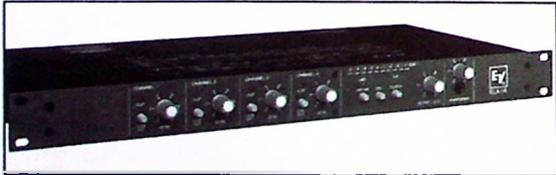
The rackmount **Electro-Voice ELX-1R** features four balanced mic/line inputs, phantom power, switchable output limiter, low cut filters, and is powered by AC or three 9V batteries. Headphone output has a separate power amp and level control and will drive any type of headphones or small a speaker. Level setting is easy with the built-in tone oscillator.
