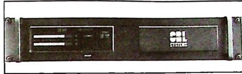
The **CRL TVS-3003** is an MTS-stereo generator and audio limiter. The TVS-3003 also has a wideband AGC providing up to 20 dB of gain reduction. The stereo generator portion of the unit is digitally synthesized and therefore is drift free. Limiting is handled by a two stage "variable transfer function" limiter which smoothly handles peak transients without generating distortion products. A "stereo enhance" feature dramatically improves your viewer's received stereo effect.
