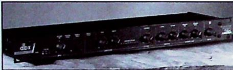
The **dbx 286A** is a mic processor with preamp, compressor, de-esser, enhancer and expander/gate combined in an affordable, compact unit. The preamp accepts mic or line level inputs, offers phantom power, an 80Hz, 18dB/Oct high pass filter plus an input level meter. An additional 1/4" TRS phone jack can accept balanced/unbalanced line signals and an insert jack between the 286A's mic preamp and signal processing sections can be used to "loop out" to external processors.
