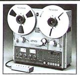
The **Tascam BR-20** has balanced +4dBm ins and outs with all major calibration controls easily accessible through the front panel. The transport is precision servo controlled for smooth operation and accurate real time counter readings. It has a ±12% pitch control, direct time locate, built in monitor speaker (optional on the BR-20T), three DC motors, a parallel remote port, three presettable
