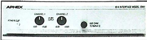
The **Aphex Model 124A** is a -10dBv to +4 or +8 dBm interface for linking consumer type equipment to professional equipment. The 124A fits in a half rack space.
