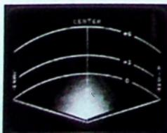
The **B&B Imagescope™** half-rack unit, is the ideal tool for any stereo audio monitoring application. It displays the complex stereo audio signal, showing the dispersion of energy as it will sound in a typical listening environment. The Imagescope™ is used to position, any track or tracks in the stereo image. At a transmission site the scope will show mono compatibility of stereo program material and allow you to observe the separation, balance and level of the stereo signal. 3U
