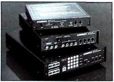
The basic Comrex LXT/R one line frequency extender system works with a standard dial telephone line or a cellular telephone to pass 250Hz of additional low frequencies. This results in more natural sounding audio, eliminating the "tinny" telephone sound. The LXT/R combines the function of an encoder and a decoder - the choice is made by pushing a single switch. (An LXT/R is required at both the sending and receiving ends of the phone line.)
