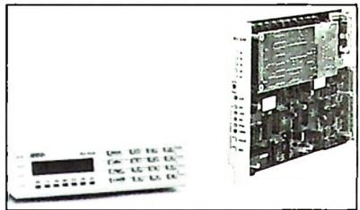
The **Adtran DSUIIAR** is a technologically advanced, high performance data service unit (DSU/CSU). It provides an interface between Digital Data Service (DDS), Basic Data Services, 4-wire Switched 56, and the customer's data terminal (DTE). The DTE interface can be selected as either RS-232 or V.35 for all data rates.
