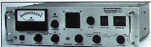
The **Delta SM-1** Splatter Monitor measures the level of splatter or any other spurious emissions which fall between 1kHz and 100kHz away from both sides of the carrier. While normally installed in an equipment rack and fed with the transmitter or common point RF sample, it also operates in the field from a twelve volt DC source fed by an optional active antenna. This portability is very useful for investigating interference complaints.
