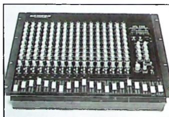
The **Samson MPL 2242** is a 22-channel, 4-buss, rack mountable mixer. It has 22 total inputs, (10 XLR balanced featuring a low-noise, padless preamp design, and 6 1/4" TRS stereo inputs). Other features include: 4-band EQ • 4 stereo aux returns • 6 aux sends, (1 pre- and 5 post-fader) • 4-bus design (using 4 dedicated group faders for submixing) with discrete group and main summing outputs • and more.
