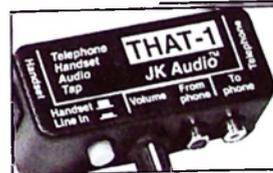
Connect **JK Audio THAT-1** between your telephone and handset jack to record or play tapes down the telephone line. A handset/line in button enables you to either talk or play a recording down the phone line without changing
