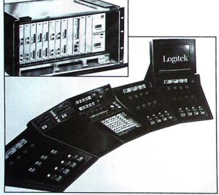
Logitek's Serial Sound System consists of a 12-slot mainframe which can hold up to eight, 8x8 mono/4x4 stereo analog or digital I/O cards, two DSP audio processor cards, two communications processor cards and up to two power supplies. The mic pre-amp unit is housed externally and offers four independent pre-amps with balanced I/O on XLR connectors.
