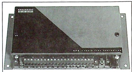
The **Broadcast Tools Audio Fade Controller** provides a convenient means of fading stereo audio. The AFC accepts stereo balanced or unbalanced audio with levels ranging from -15dB to +10dB. The output is balanced and may be adjusted from -20dB to 10dB. The AFC is equipped with preset parallel inputs and eight node serial port.
