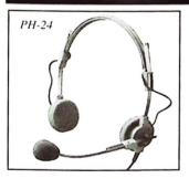
The **Telex PH-24** has a full studio quality electret condenser microphone sound plus lightweight comfort. The PH-24 miniature noise cancelling electret microphone provides an extremely flat frequency response with significantly attenuated background noises and comes with a push to cough switch. Earphones  $150\Omega$  with a 9' cord to pigtail.
