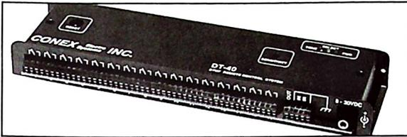
The **Conex DT-40** DTMF Tone Remote Control System accepts DTMF tones from an audio line, receiver, or other source. After giving your user access code, it allows remote control of sixteen SPDT relays. The relays can be momentary, latching, or interlocking. A switch-selectable device selection code allows up to 15 DT-40's to be individually controlled from one audio source. It has miniature screw-clamp terminal strips for easy connection.
