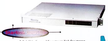
A 2.4 GHz Spread Spectrum link for stereo remotes up to distances of 25 miles.
