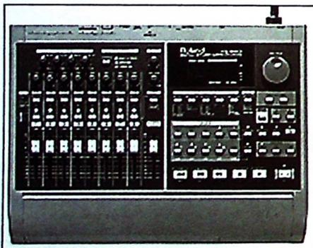
recorder, a digital mixer and studio-quality multi-effects (an add-on board option) in a completely self contained unit.
