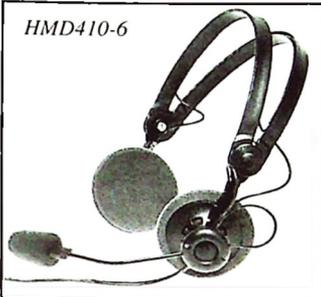
The **Sennheiser HMD410-6** is a supraural, open-air, 600Ω headphone (20-18kHz) with a dynamic supercardioid, 200Ω boom mic (50-12kHz). Comes supplied with a 6' stranded steel cable terminated in stripped and tinned leads. Weight 18 oz.
