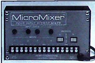
**Henry's Micromixer** will accept up to four balanced or unbalanced line-level inputs and will mix them to a stereo output. A level control for each input provides adjustment from "off" to +10db of gain. "Micro-Assign" switching permits each input to be assigned to the left, right, or both
