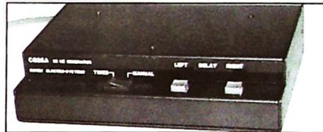
The **Conex CS-25B** is a compact and modular 25 Hz tone sensor for use in broadcast automation, tape control, or remote signaling systems. The sensor detects 25 Hz sub-audible tones that typically signal the end of a program selection. The resulting relay contact closures can be used to start the next source and stop the current source. A stereo high-pass filter module is offered as an option to provide absolute protection from program tripped cues.
