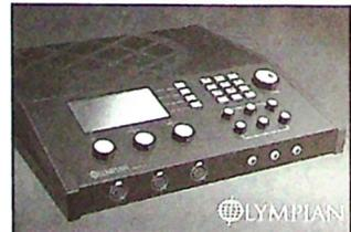
Olympian™ is a portable, stereo ISDN codec/mixer with memory for full duplex bi-directional operation. It contains MUSICAM®, Layer II, Layer III, G.722 & G.711 algorithms, plus hybrid interface for direct connection to an analog telephone line. Three headphone outputs, each with separate send and return level controls, 256 speed dial addresses, plus storage for multiple venue terminal adapter configurations. Olympic Memory Snap Shot—OMSS™—smart preset lets you save all parameters.
