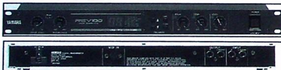
The **Yamaha REV 100** is basically a no-fuss signal processor — all you have to do is select one of its 99 preset effects and play. The three most critical parameters for all effect programs are adjustable via rotary panel controls — just rotate the appropriate controls until the sound is right. REV 100 effect categories include: reverb, true stereo reverb, gate
