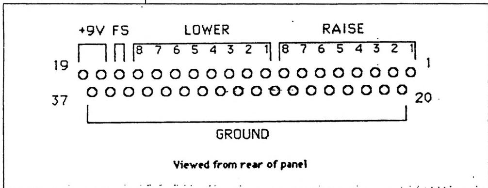
figure 3-2 Rear Panel Control Output Connections
