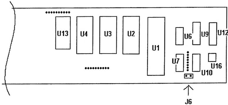
Cut the link between the two pins of J6. Add a jumper to connect pins 1 and 6 of the baud rate selector for 1200 baud. Note: Pin 1 is the pin closest to J6.
