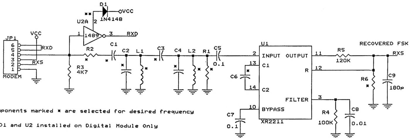
Components marked \* are selected for desired frequency
