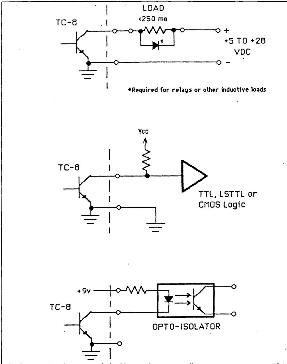
figure 3-4. Output Connections to External Devices.
