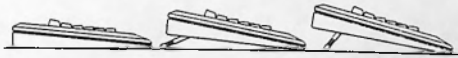
Keyboard adjusts to three height levels. Available in French, German and U.K. configurations.
