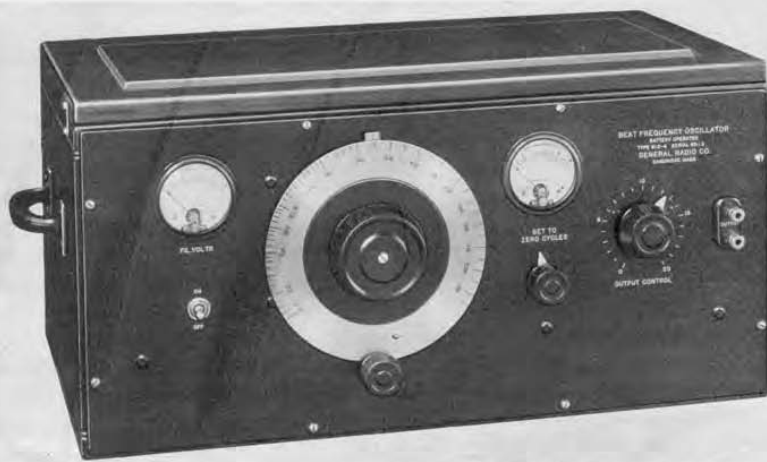
The TYPE 613-A Beat-Frequency Oscillator is operated from batteries inside the cabinet
