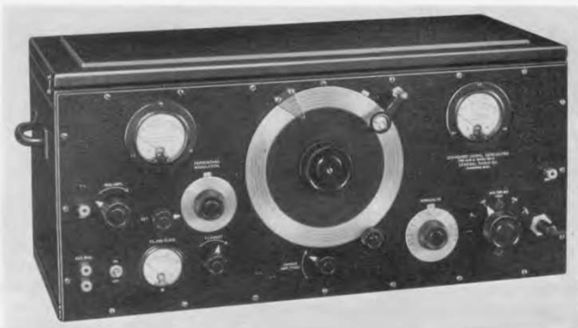
The main tuning control for the TYPE 603-A Standard-Signal Generator carries a dial with 600 divisions. The microscope at its right is an aid in making close settings; the triangular index at the left is for use with calibrations filled in with pencil by the user.
