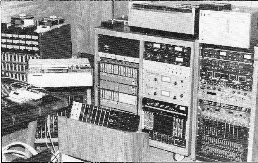
The two digital audio processors — dbx Model 700 and Sony PCM-1610, plus companion U-Matics — used for comparison evaluations at Crescendo.
