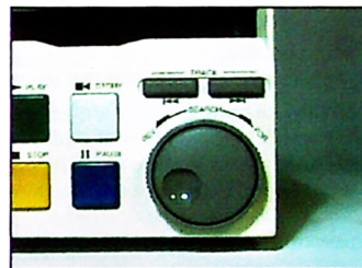
Jog Shuttle for Quick Frame Search & Location
