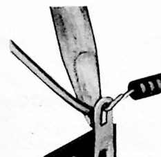
3. Apply solder BETWEEN iron and connection
