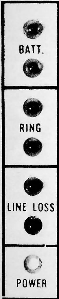
**BATT:** THESE TWO AMBER LEDS WILL ALTERNATELY FLASH TO WARN YOU THAT THERE IS ONLY A COUPLE OF HOURS OF BATTERY LIFE LEFT. TO CONSERVE BATTERY LIFE WHEN THERE IS NO EXTERNAL POWER AVAILABLE YOU MAY SHUT DOWN THE CLOCK AND TIMER DISPLAYS WHEN THEY ARE NOT NEEDED (EACH CLOCK AND TIMER DISPLAY CONSUMES APPROXIMATELY 80 MA.)
