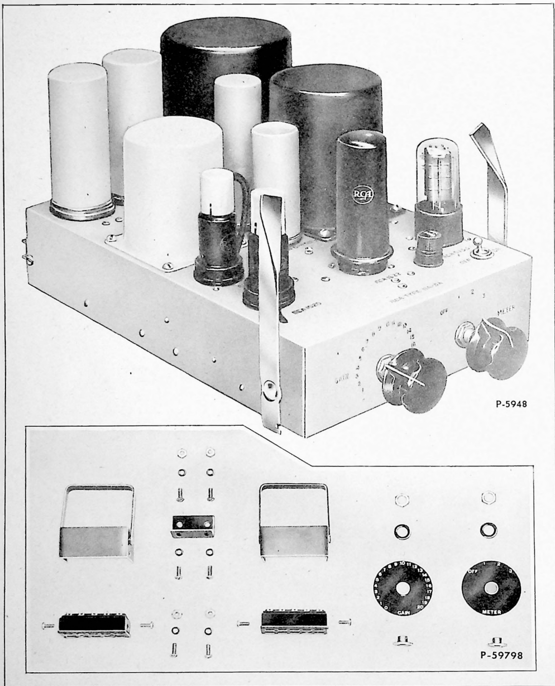
Figure 1—Front view of Type BA-3A Program Amplifier. Inset: Adapter kit supplied with amplifier.
