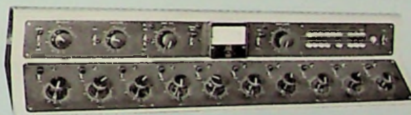
Custom audio control console designed and built for Station KHJ's television studio. It includes complete mixing and cueing facilities for five microphones and an announce microphone, two turntables, one remote and three utility inputs.
