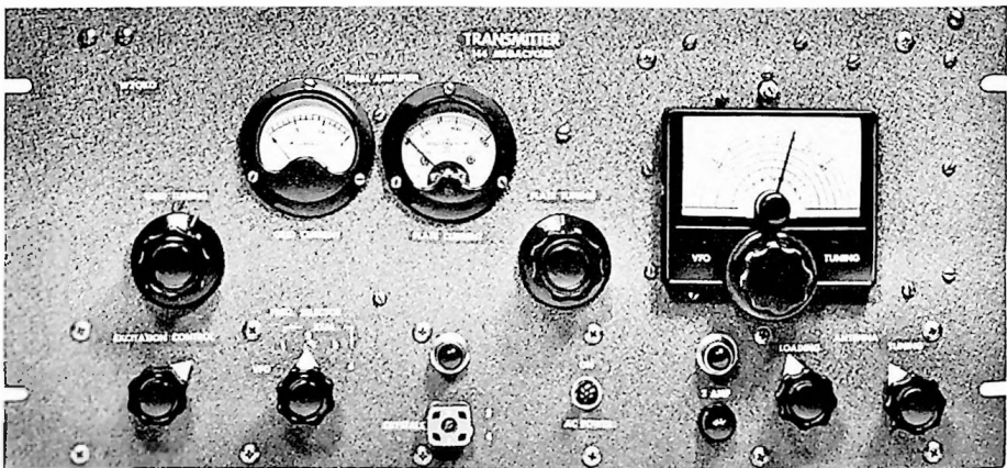
Figure 1. Panel view of the 144-Mc transmitter. VFO bandset control is directly above the center of the VFO dial.
