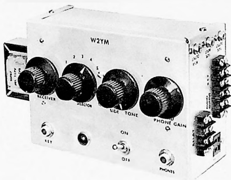
Figure 1: The W2YM magnetic-tape keyer control, or "Keyer." All components are contained within a 7-by-5-by-3-inch minibox with the exception of the power transformer.
