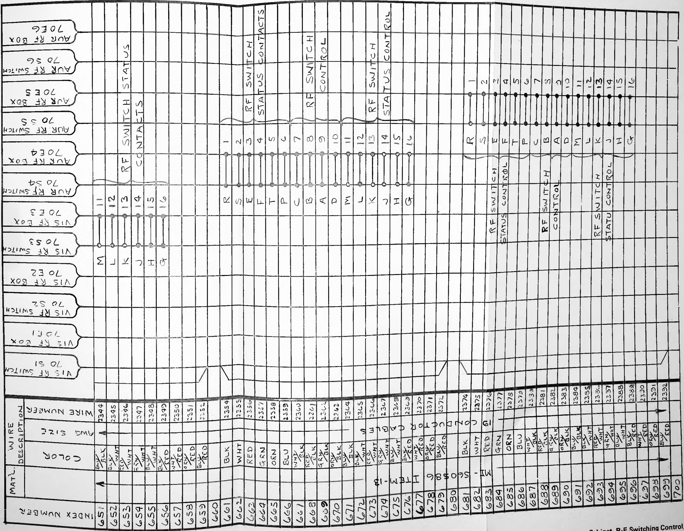
Figure 4. TT-30FL Inter-Cabinet, R-F Switching Control, and Remote Control Interconnection Wire Chart - 3732114 (Sheet 14 of 24)
