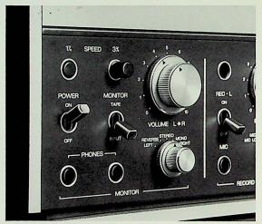
Externally the B77-LS differs only in that its speed selector buttons are labelled 1% and 3% ips. The capstan motor runs at a reduced number of rpm and it is equipped with a thinner capstan shaft
