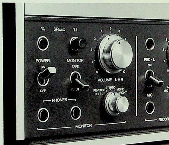
Externally the B77-SLS differs only in that its speed selector buttons are labelled  $15/16$ – $17/8$  ips. The capstan motor runs at a reduced number of rpm and it is equipped with a thinner capstan shaft.
